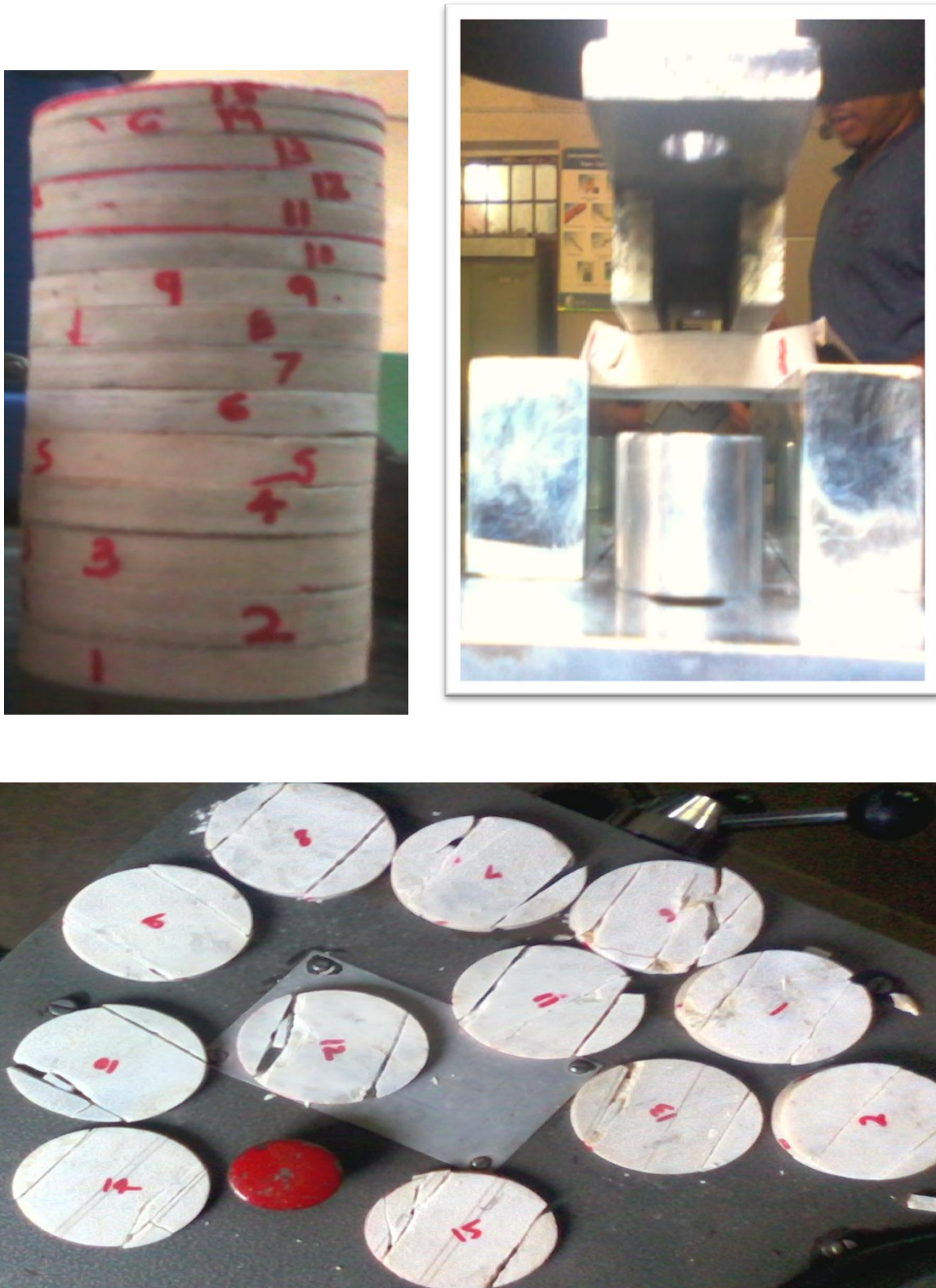
Fig. 3.2 The specimen before, during and after testing
