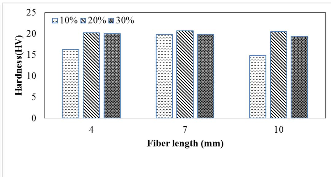
**Figure 4.4** Effect of fiber parameters on hardness of composite
