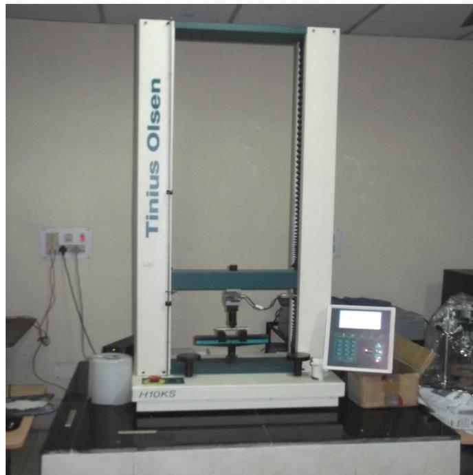
**Figure 3.2** Experimental set up for tensile and flexural test
