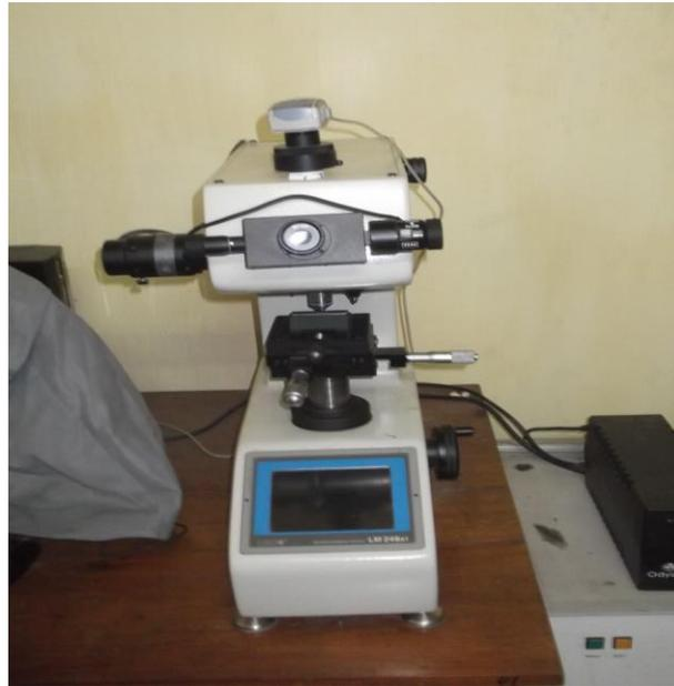
**Figure 3.3** LECO Micro hardness tester
