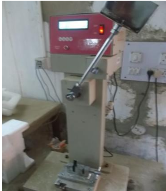
Fig: 3.6 Experimental setup of impact test
