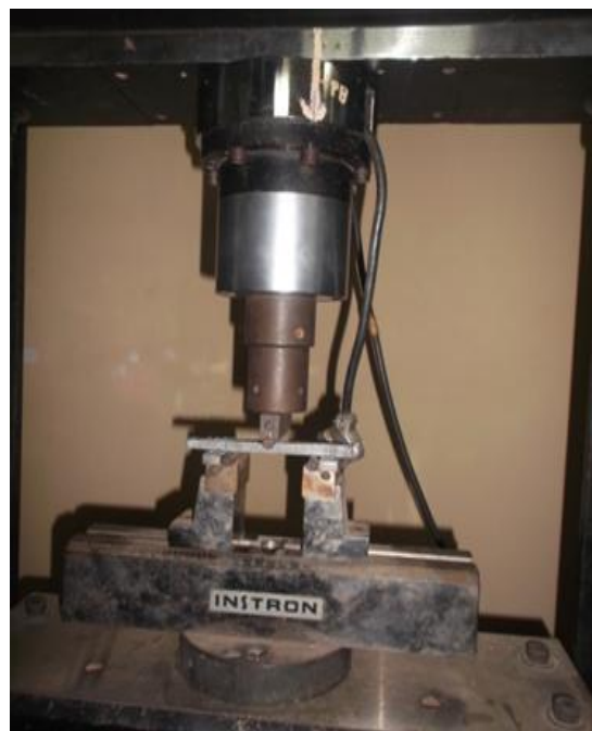
Fig: 3.5 Loading arrangement for flexural test
