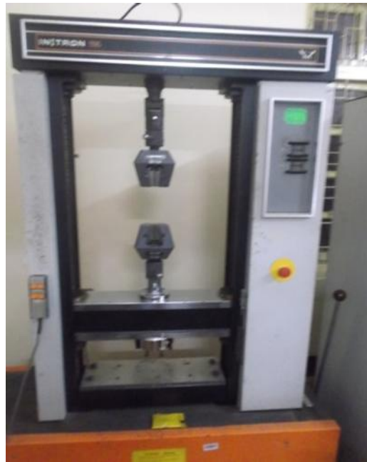
Fig:3.3 Experimental set up of tensile test
