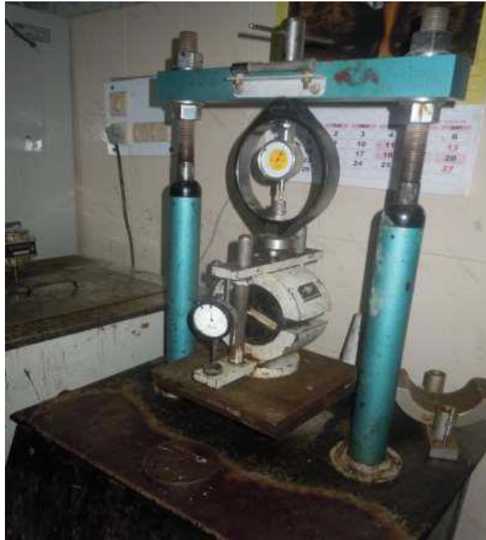
FIG 11: Marshall Test Machine
