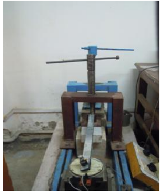
Figure 5.3: Beam is arranged on frame for fixed-fixed and cantilever conditions
