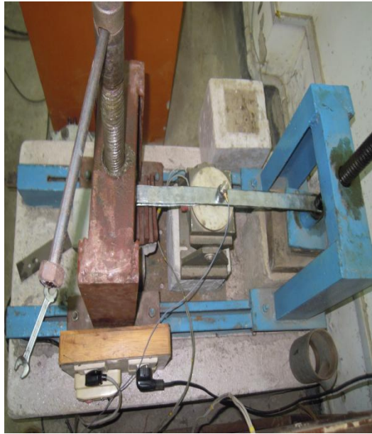
Figure 5.3: Beam is arranged on frame for fixed-fixed and cantilever conditions
