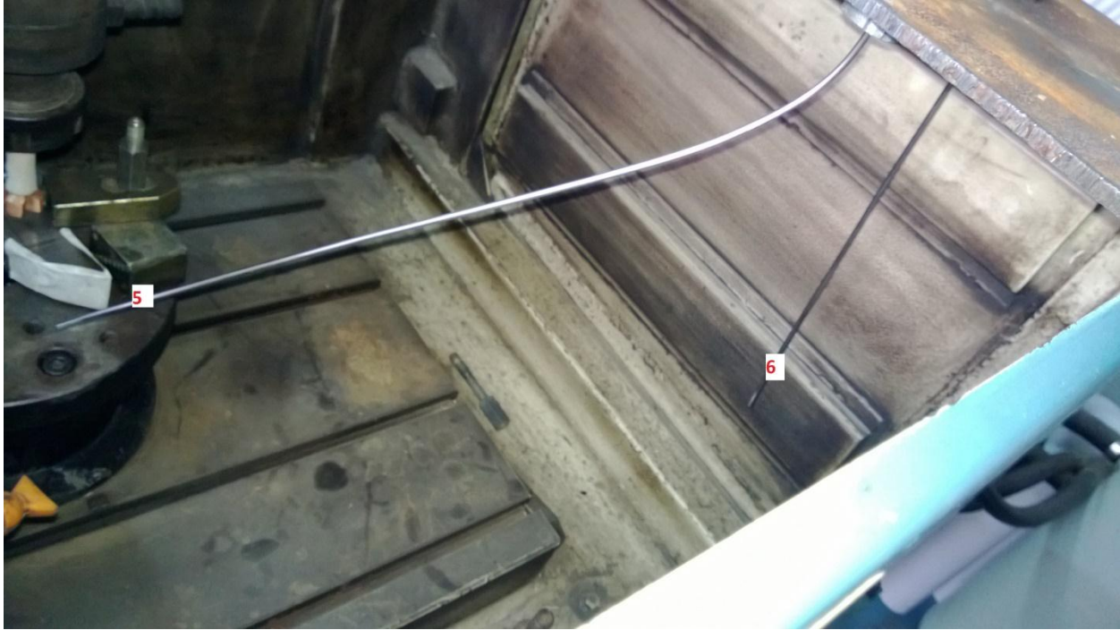
Fig.8. placing of thermocouple 5 and 6 in dielectric.
