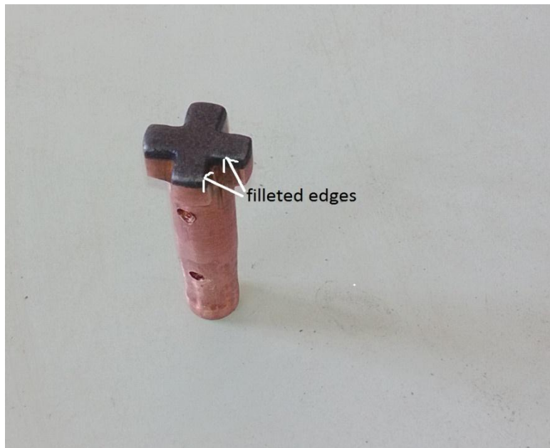
Fig.24. figure showing the filleted edges due to more material removal at periphery.
