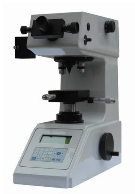
**Fig6.2: Micro-Hardness Tester**
