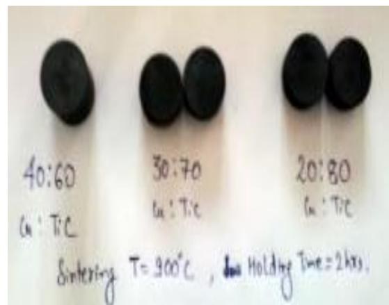
**Fig5.2: Top view of compacted tool**
