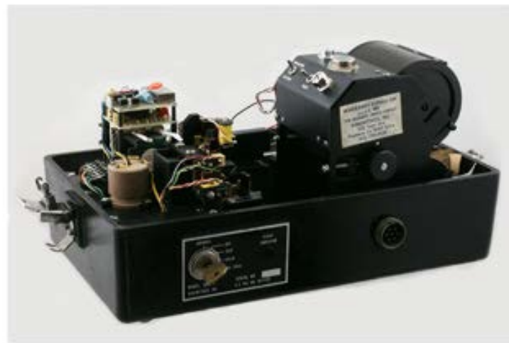
Figure 4.1: Accelerograph, courtesy of Museum of Geostrophysics National Observatory of Athens [37]
