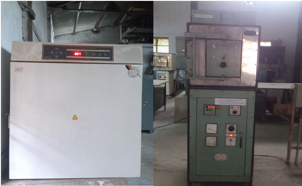
Fig: 2. Dryer machine and Heating Furnace
