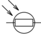
A light-dependent resistor (LDR) is a light controlled variable resistor. It exhibits photoconductivity, as the incident light intensity increases, the resistance of a LDR decreases. A LDR can be applied in a light sensitive detector circuit [17]. We have used the LDR for a similar purpose in our robot circuit.
