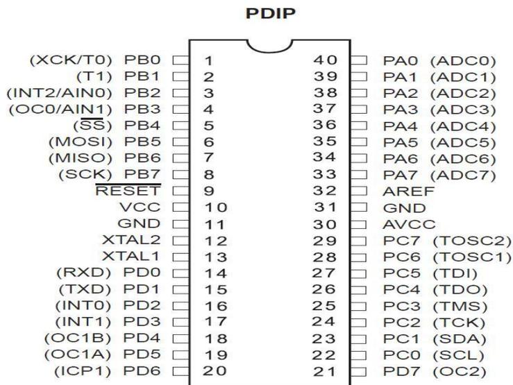
Figure 3.8 Pin Diagram of ATmega 32 microcontroller
