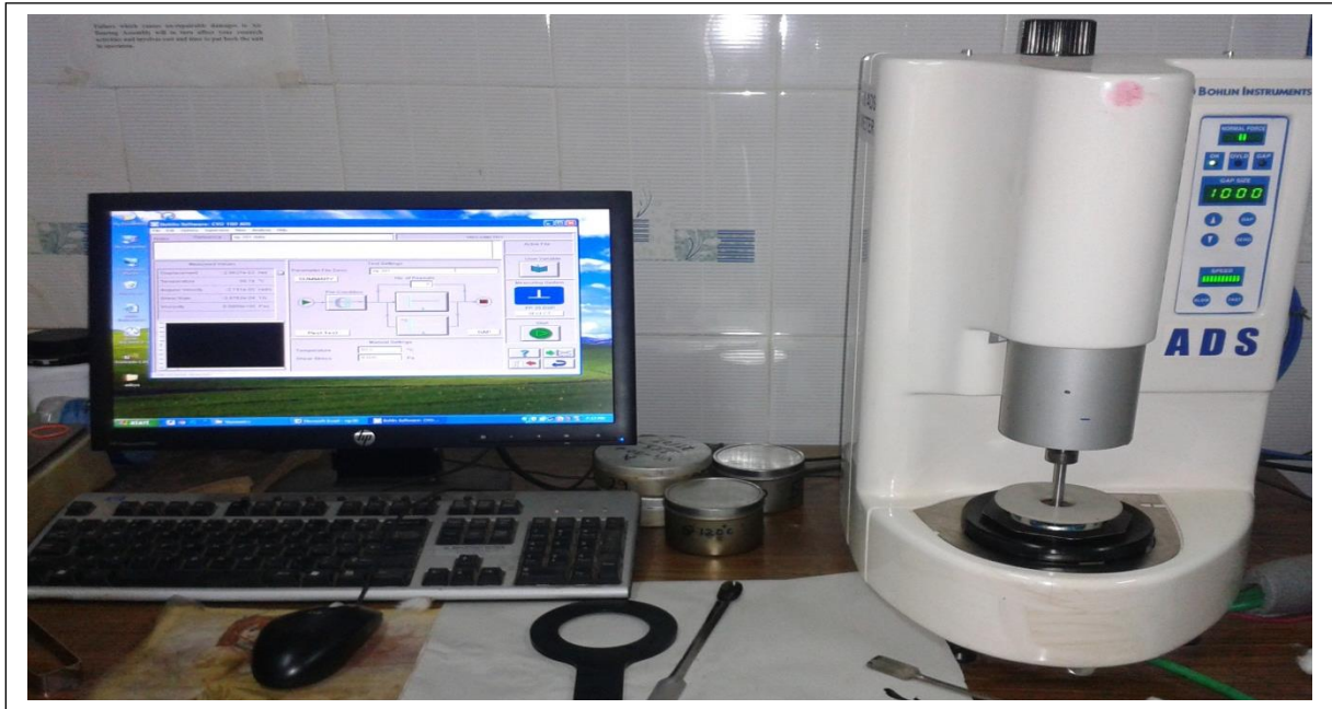
Figure 3.3: Showing Stress Controlled Dynamic Shear Rheometer (DSR)
