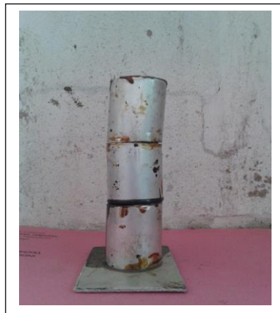
Figure 3.18: Tube used in storage stability test.
