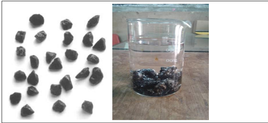
Figure 3.17: Stripping test of aggregate test through boiling test.
