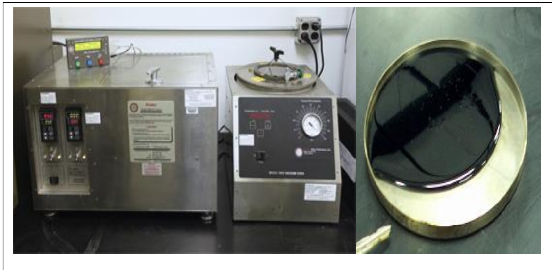
Figure 3.12: PAV with degasser and pan for sample storage [www.pavementinteractive.org]
