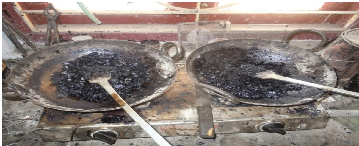
Fig4.Preparation and mixing of SMA during experimentation process.
