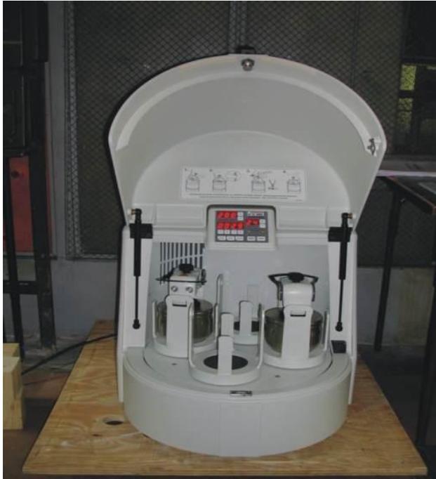
Fig 2 – Planetary Ball mill
