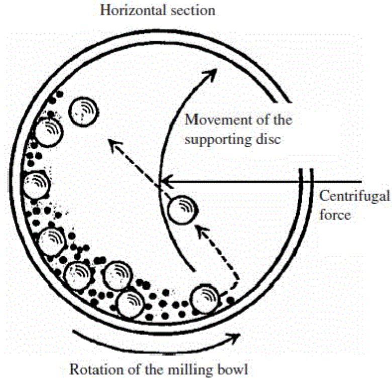
Fig 1 – Movement of milling bowl and balls
