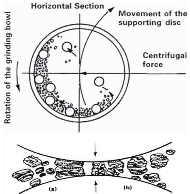
Fig – 3 Milling mechanism
