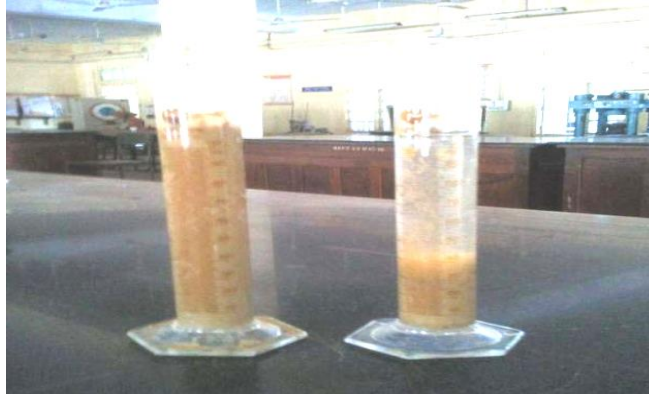
Figure 3.6 Free swell test for soil
