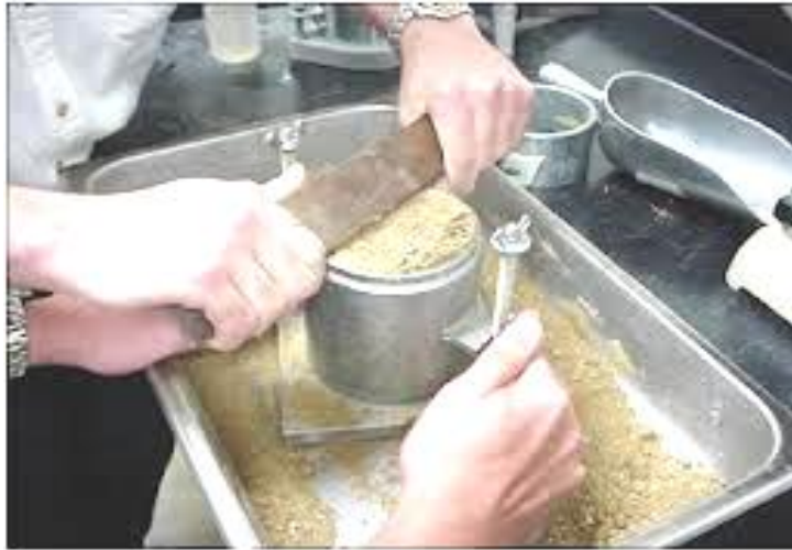
Figure 3.8 Compaction test for soil
