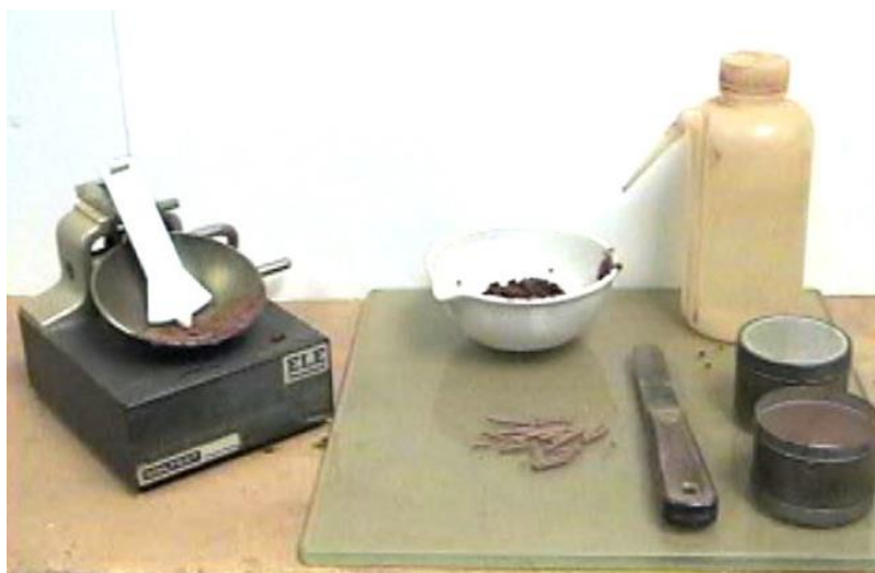
Figure 3.5 Liquid limit and plastic limit test for soil
