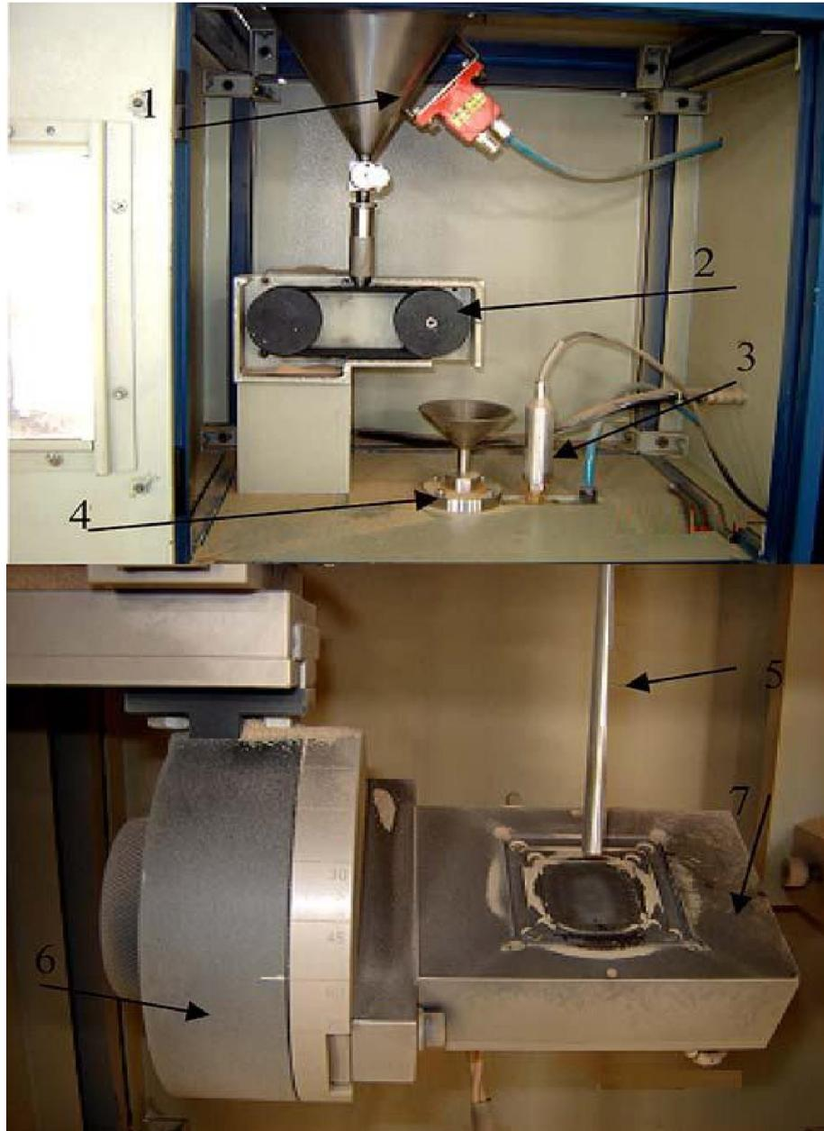
**Figure-6.1** Details of erosion test rig. (1) Sand hopper, (2) Conveyor belt system for sand flow, (3) Pressure transducer, (4) Particle-air mixing chamber, (5) Nozzle, (6) X-Y and h axes assembly, (7) Sample holder.
