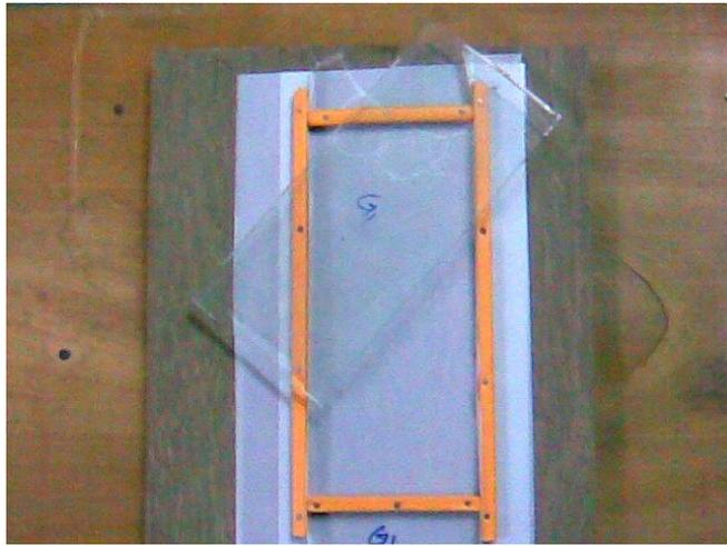
Figure-3.7 Mold used for composite preparation
