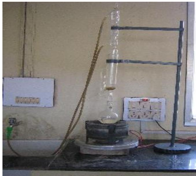
Figure-3.1 Soxhlet Extractor
