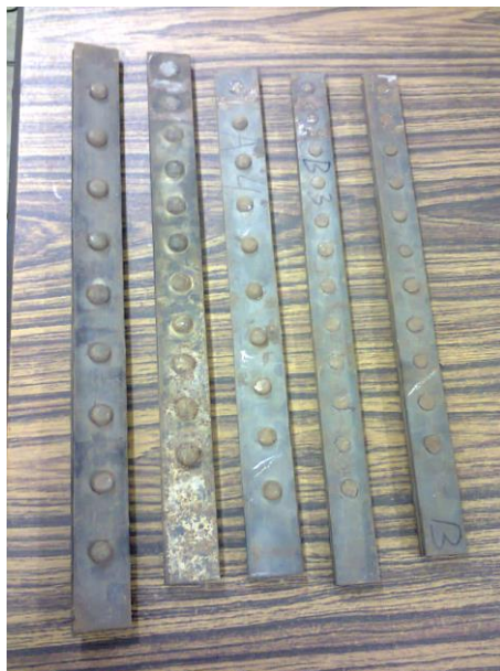
Figure 5.4 Photograph of the riveted mild steel specimens
