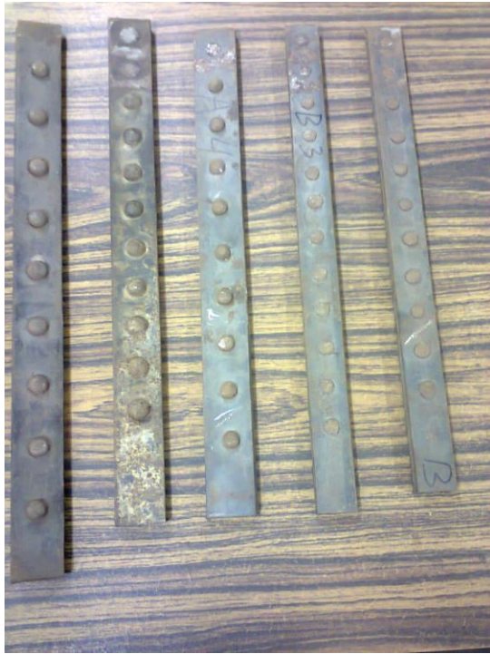
Figure 5.1 Photograph of the thin riveted mild steel specimens
