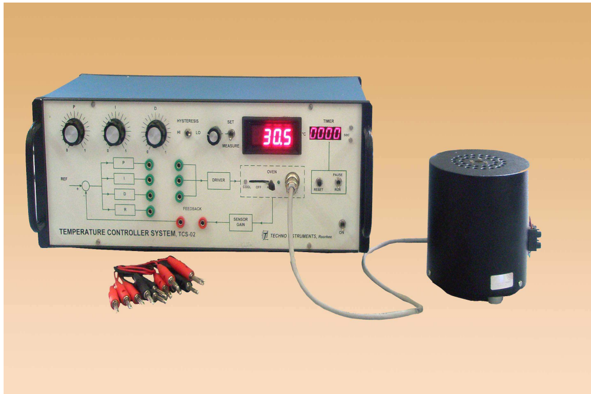
Figure 2.2: Temperature control plant laboratory setup
