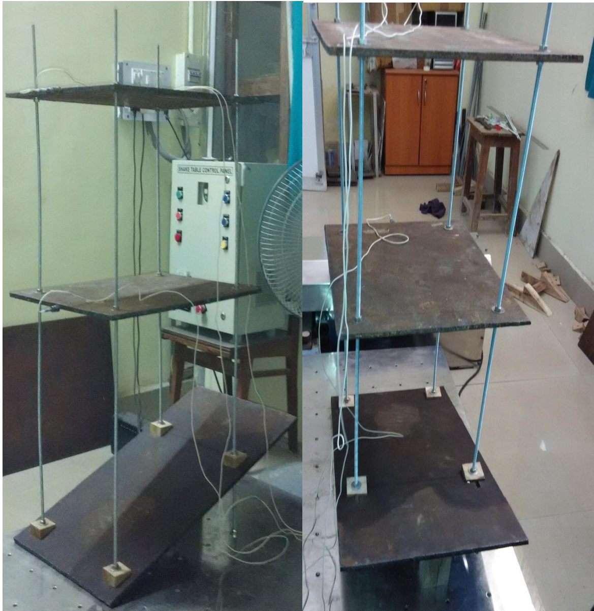
Figure 3.7: Experimental Model for 20° slope
