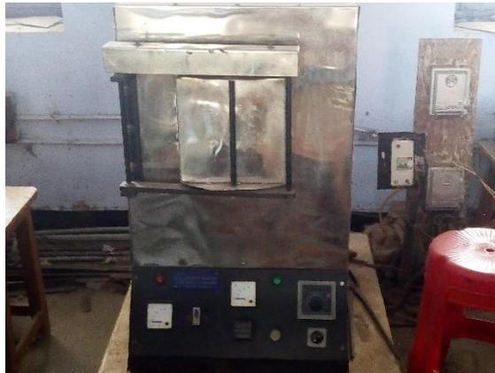
*Figure 5-A muffle furnace*
