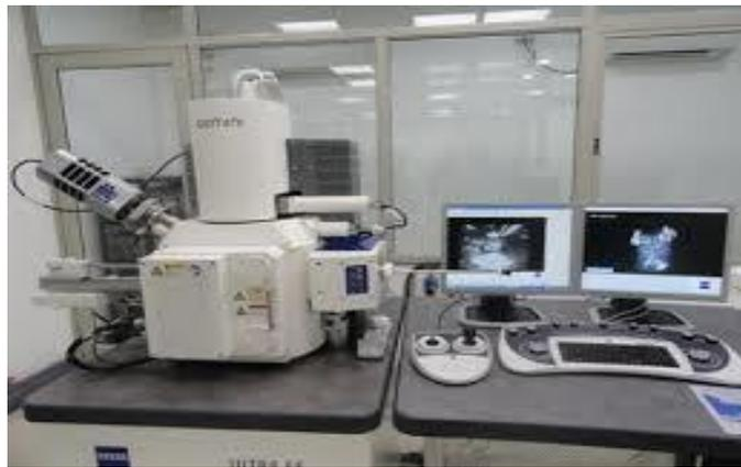
Figure 8.-A typical FESEM set-up/SEM
