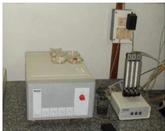
Figure 10- A standard Differential Scanning Calorimetry Set-up
