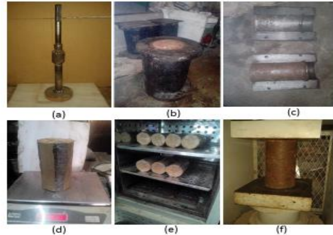
Figure 3.4. Sequences involved in preparation and testing of UCS of cylinder specimens (a) Tamper used with vibratory hammer for compaction of cylindrical specimens, (b) Cylindrical mould (101.6 mm diameter and 203.2 mm height) used for compaction, (c) Removal of specimen from the mould after 24 hours, (d) Weighing of specimen after proper sealing, (e) Curing of specimens in the BOD incubator at a constant temperature ( 23 \pm 1.7^\circ\text{C} ) (f) Unconfined compression test of specimen (after 7 days) using a Compression testing machine.
