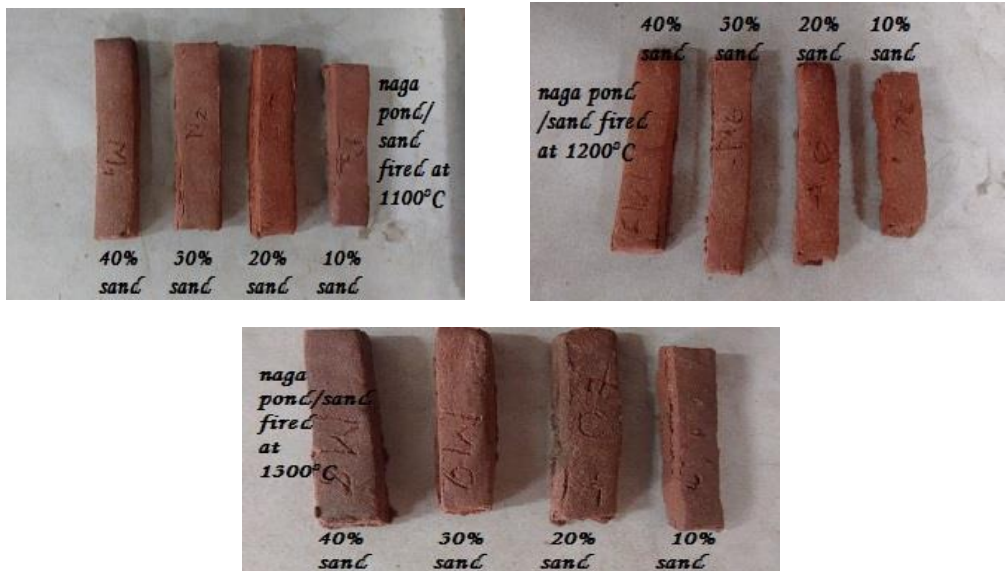
Figure 3 Naga Pond Clay-Sand bricks fired at 1100°C, 1200°C and 1300°C
