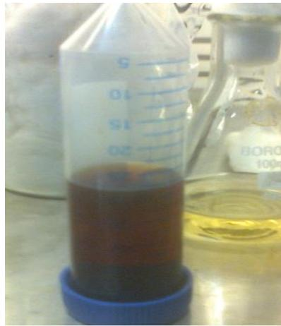
Graphene oxide NPs prepared by Pyrolysis method
