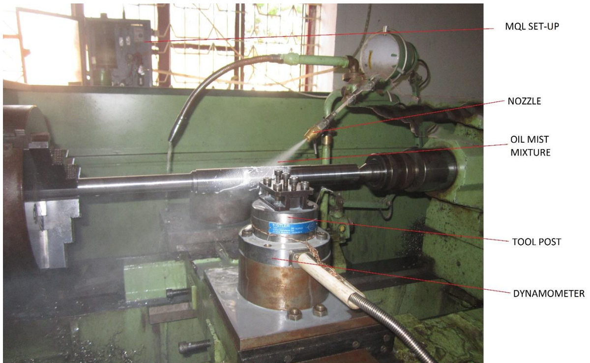
Figure 3.2: Experimental set-up for MQL lubrication system
