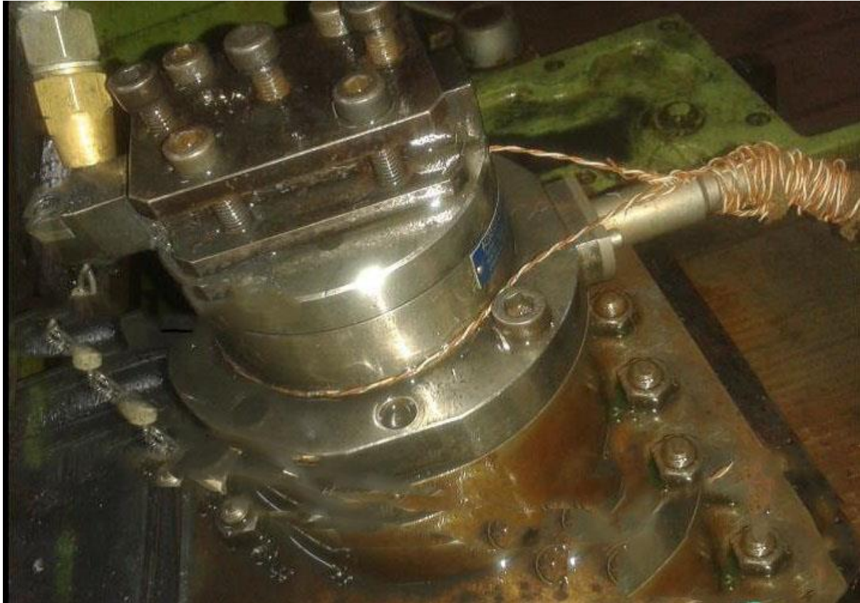
Figure 3.4: Dynamometer for cutting forces measurement
