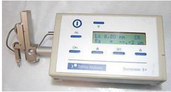
Figure 3.5: Talysurf or Profilometer for surface Roughness measurement
