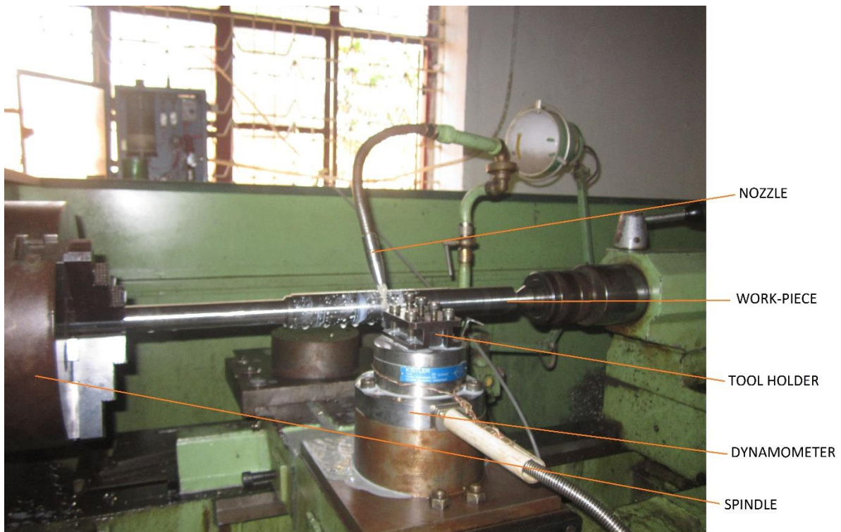
Figure3.1: Experimental set-up for conventional cooling.
