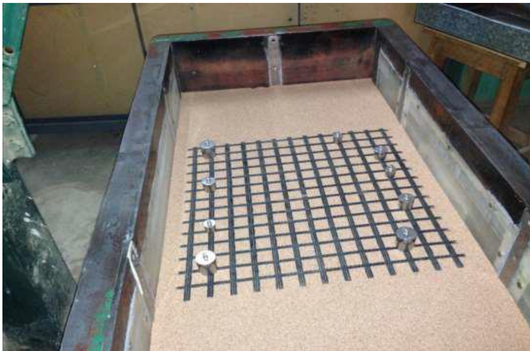
Fig 4.2 placement of geogrid in the tank
