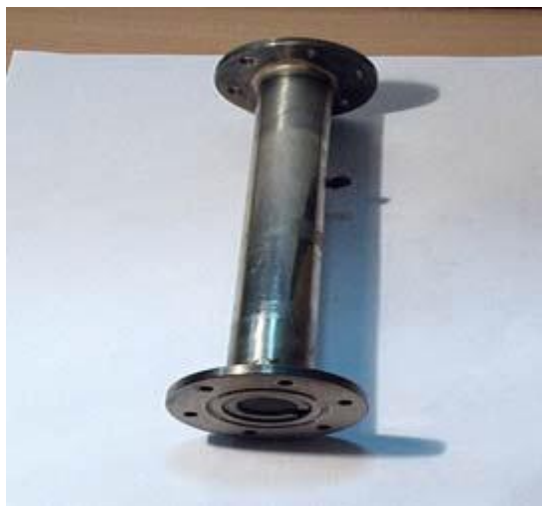
Figure5. Figure of Regenerator
