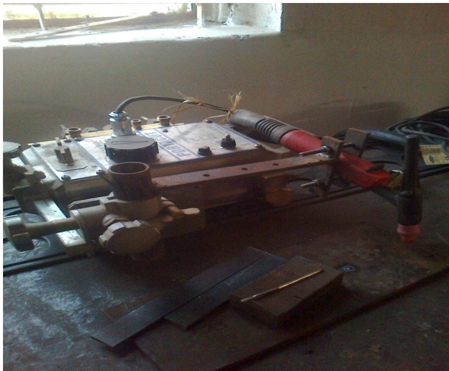
Fig.4: TIG Torch with movable Tractor
