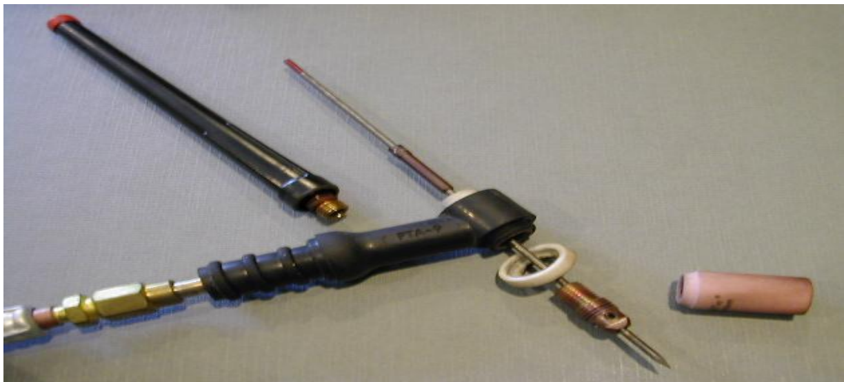
Fig.5: TIG welding torch de-assembled
