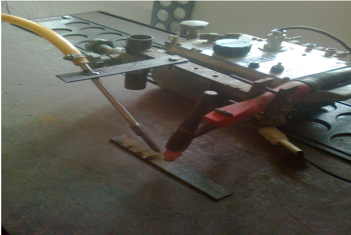
Fig.-15: Nozzle fitted to the tractor
