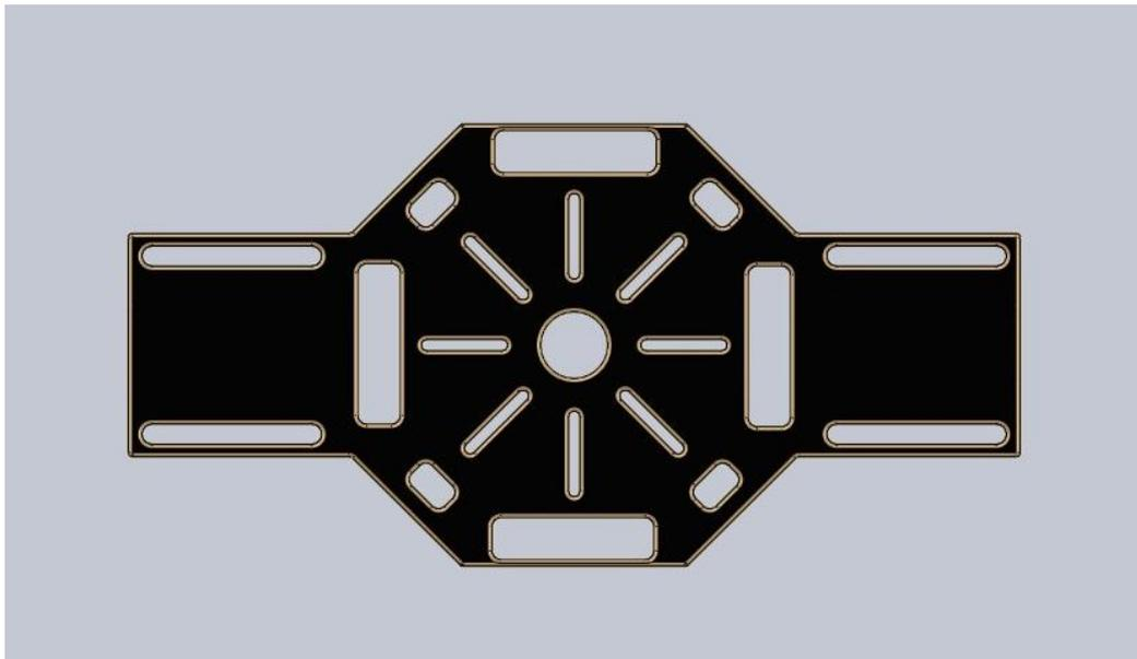
Figure 6.1: Design of Bottom Plate
