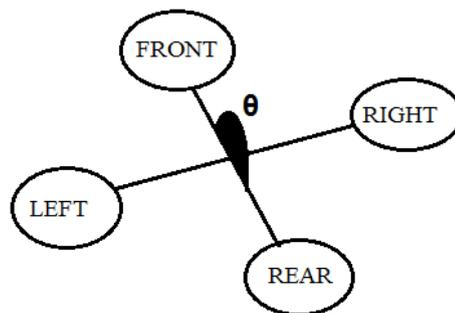
Figure 3.1: Direction of Pitch of Quadcopter
