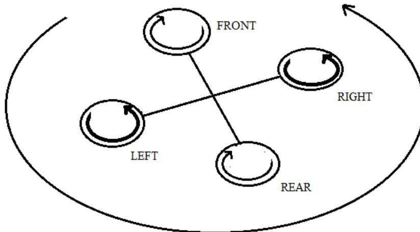
Figure 3.8: Leftward motion of Quadcopter
