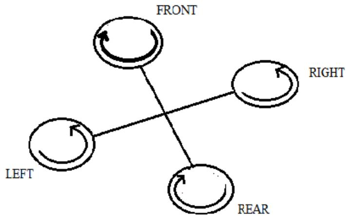
Figure 3.7: Backward motion of Quadcopter
