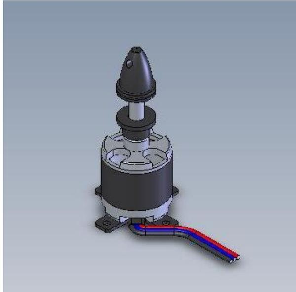
Figure 6.4: Design of Brushless DC Motor
