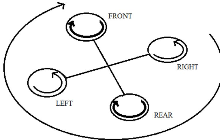
Figure 3.9: Rightward motion of Quadcopter
