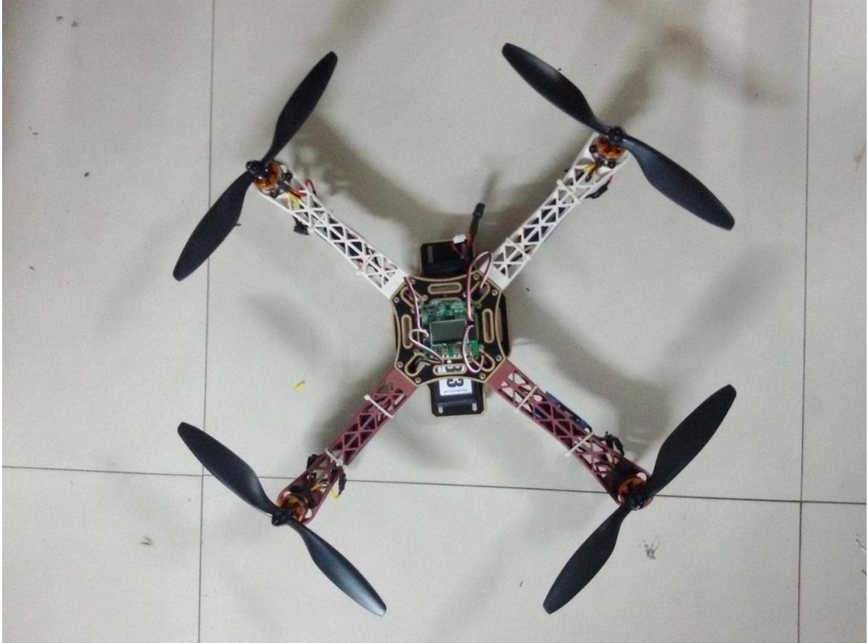
Figure 7.1: Assembled unit of the Quadcopter
