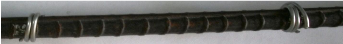
Fig 3.4: 10mm Circular [MS] rods with baffle spacing 7.5
