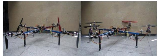
Fig. 21. Actual model showing driving and flying modes
