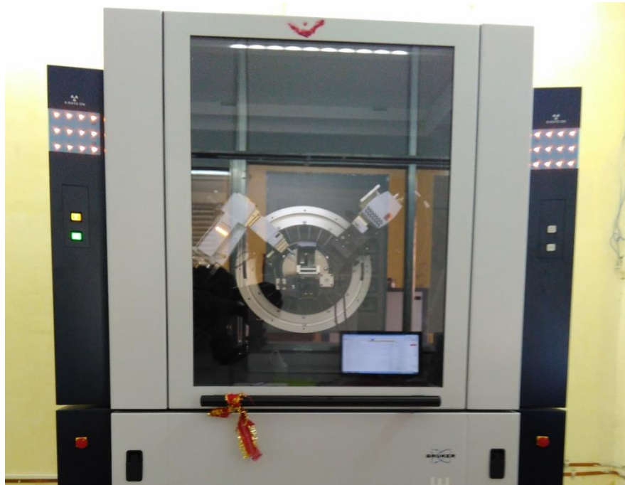
Fig.8: Set-up for XRD-texture measurement.
