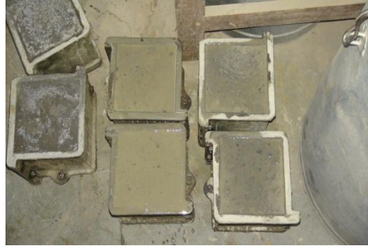
b) Concrete mix filled in mould
