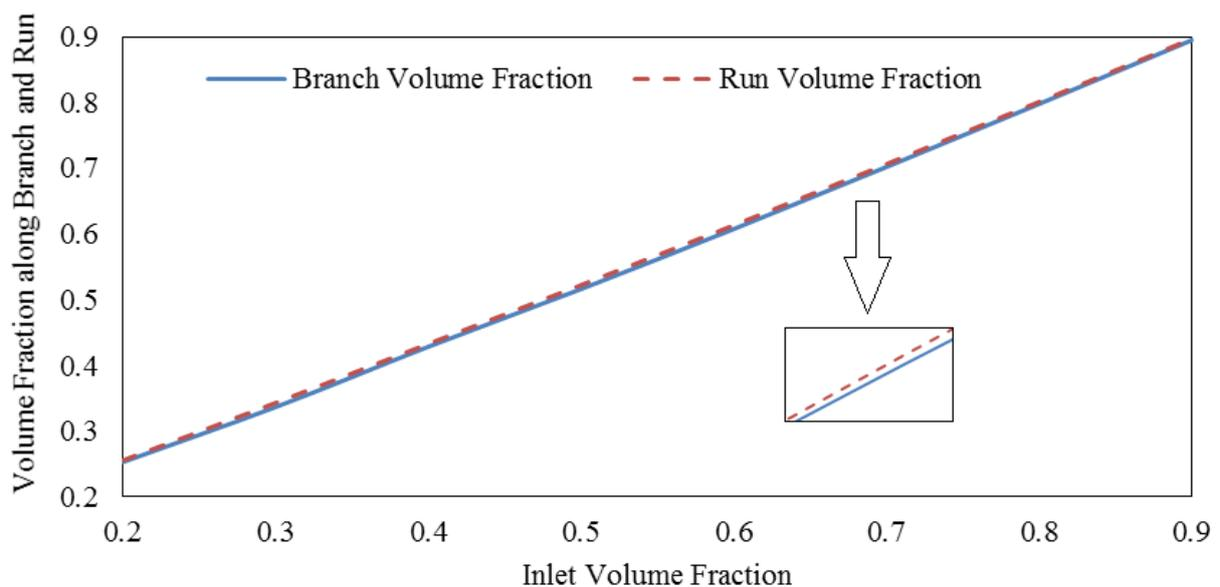
Figure 15: Effect of inlet volume fraction on branch and run volume fraction for soybean oil-water, 11 mm dia. Tee junction
