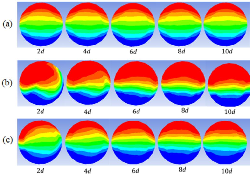
Figure 5: Phase distribution at different cross-section of (a) inlet, (b) branch and (c) run arm
