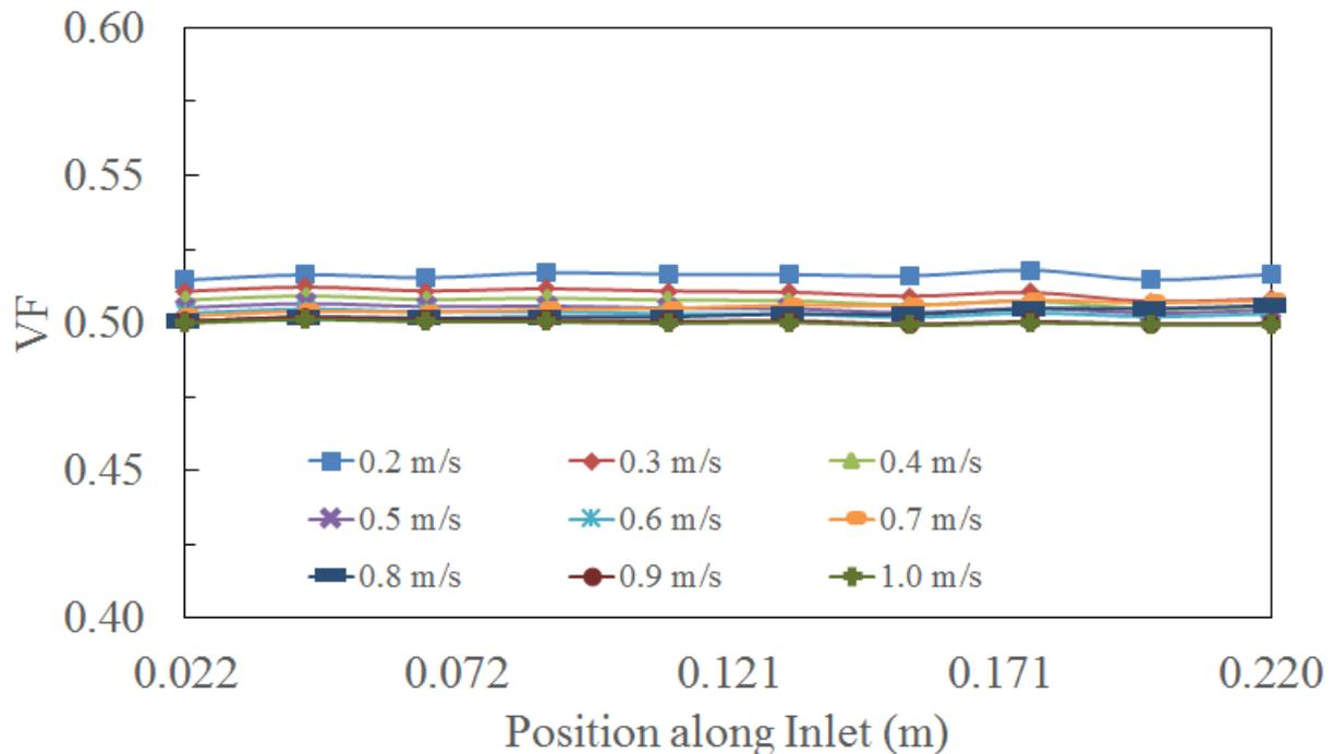
Figure 8: Variation in VF along inlet arm for diesel-water pair
