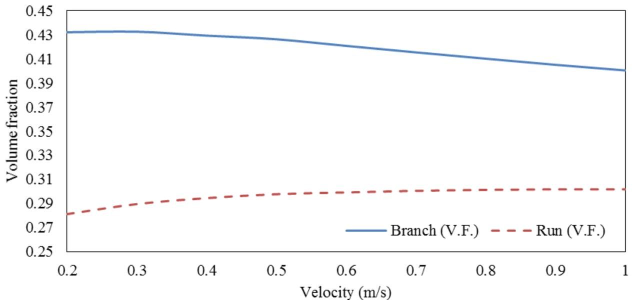
Figure 12: Effect of inlet mixture velocity for diesel-water fluid pair, 11 mm diameter Tee junction, inlet VF 0.3
