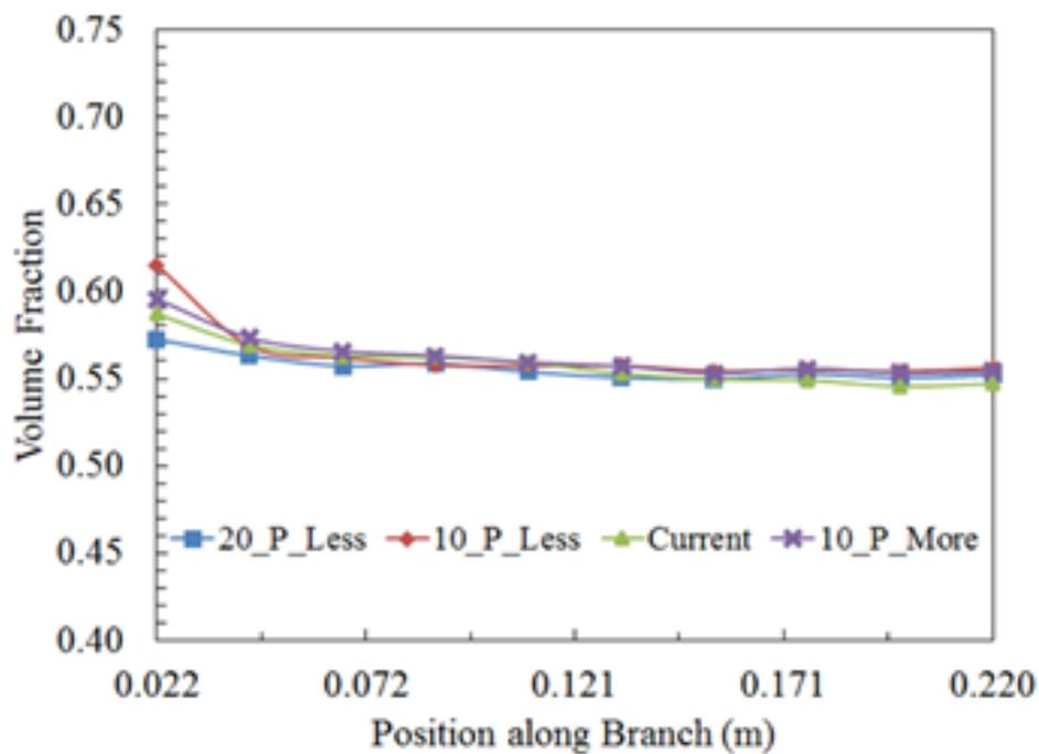
Figure 4: Volume fraction variation for different grid size along inlet and branch arm.
