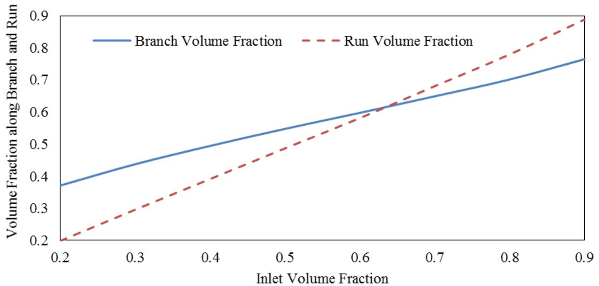
Figure 14: Effect of inlet volume fraction on branch and run volume fraction for kerosene-water, 11 mm dia. Tee junction
