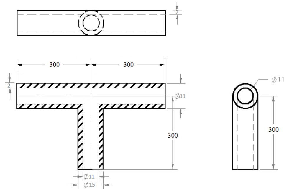
Figure 20: Design of 11 mm internal diameter Tee junction
