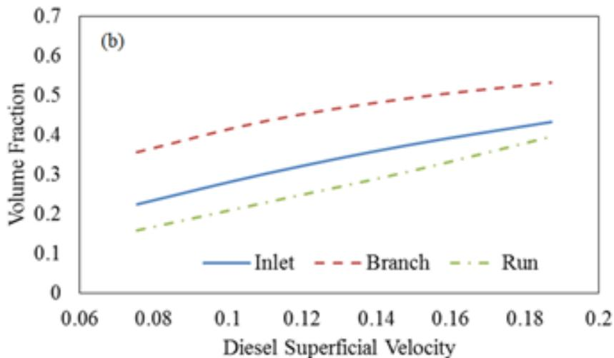
Figure 22: Effect of diesel superficial velocity on branch and run volume fraction for water superficial velocity of 0.2104 m/s
