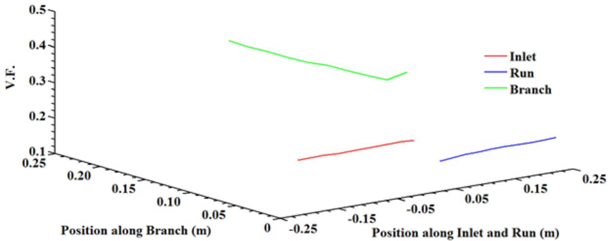
Figure 6: 3-D plot of volume fraction for inlet VF 0.2, inlet mixture velocity 0.5
