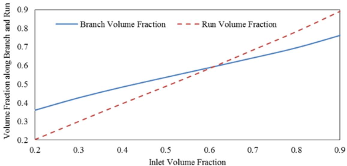
Figure 13: Effect of inlet volume fraction on branch and run volume fraction for diesel-water, 11 mm dia. Tee junction
