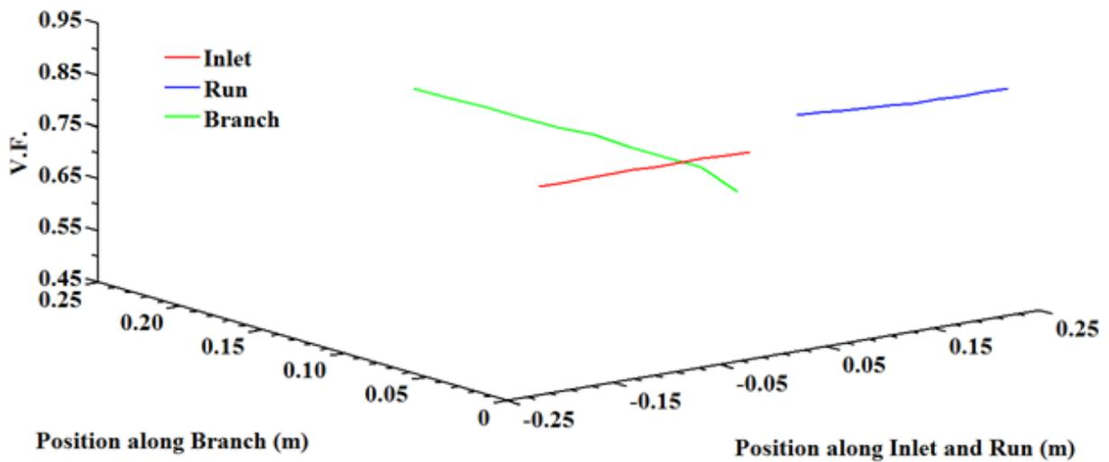
Figure 7: 3-D plot of volume fraction for inlet VF 0.9, inlet mixture velocity 0.5
