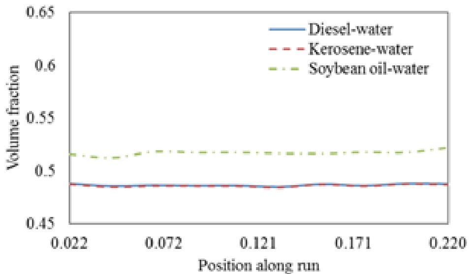
Figure 18: Effect of change in fluid pair on run arm volume fraction for 11 mm diameter Tee junction
