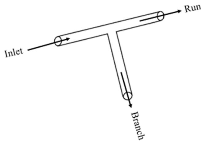
Figure 1: Schematic of a Tee junction
