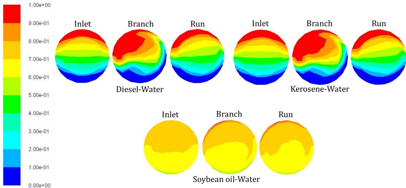
Figure 19: Phase contour for three different type of fluid pair for a fixed inlet mixture velocity and volume fraction
