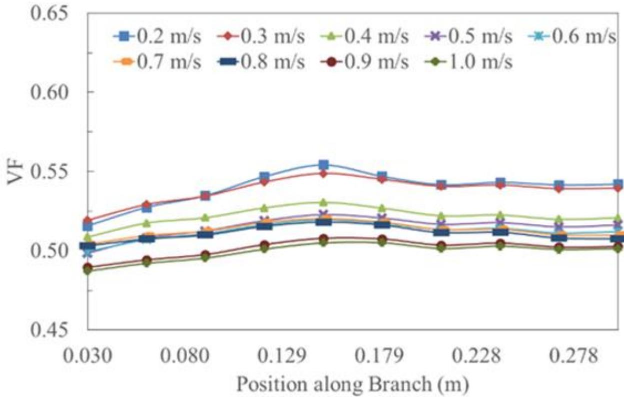
Figure 11: Variation of VF along branch arm for soybean oil-water pair
