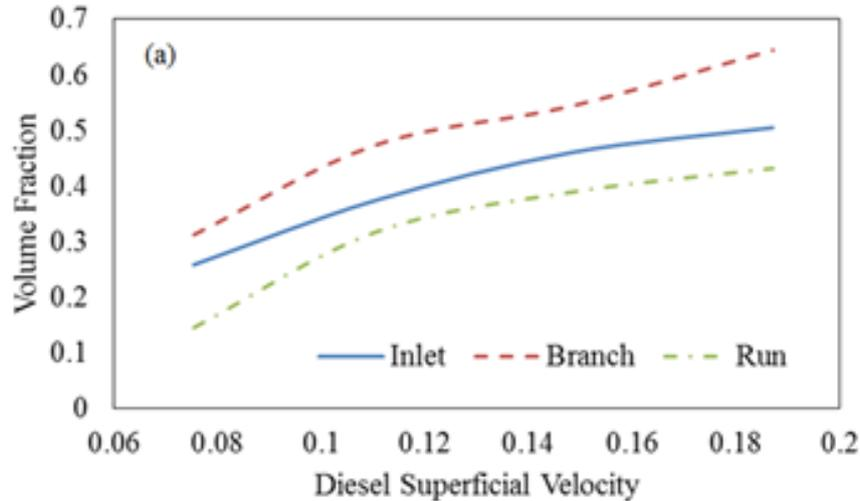
Figure 21: Effect of diesel superficial velocity on branch and run volume fraction for water superficial velocity of 0.1754 m/s
