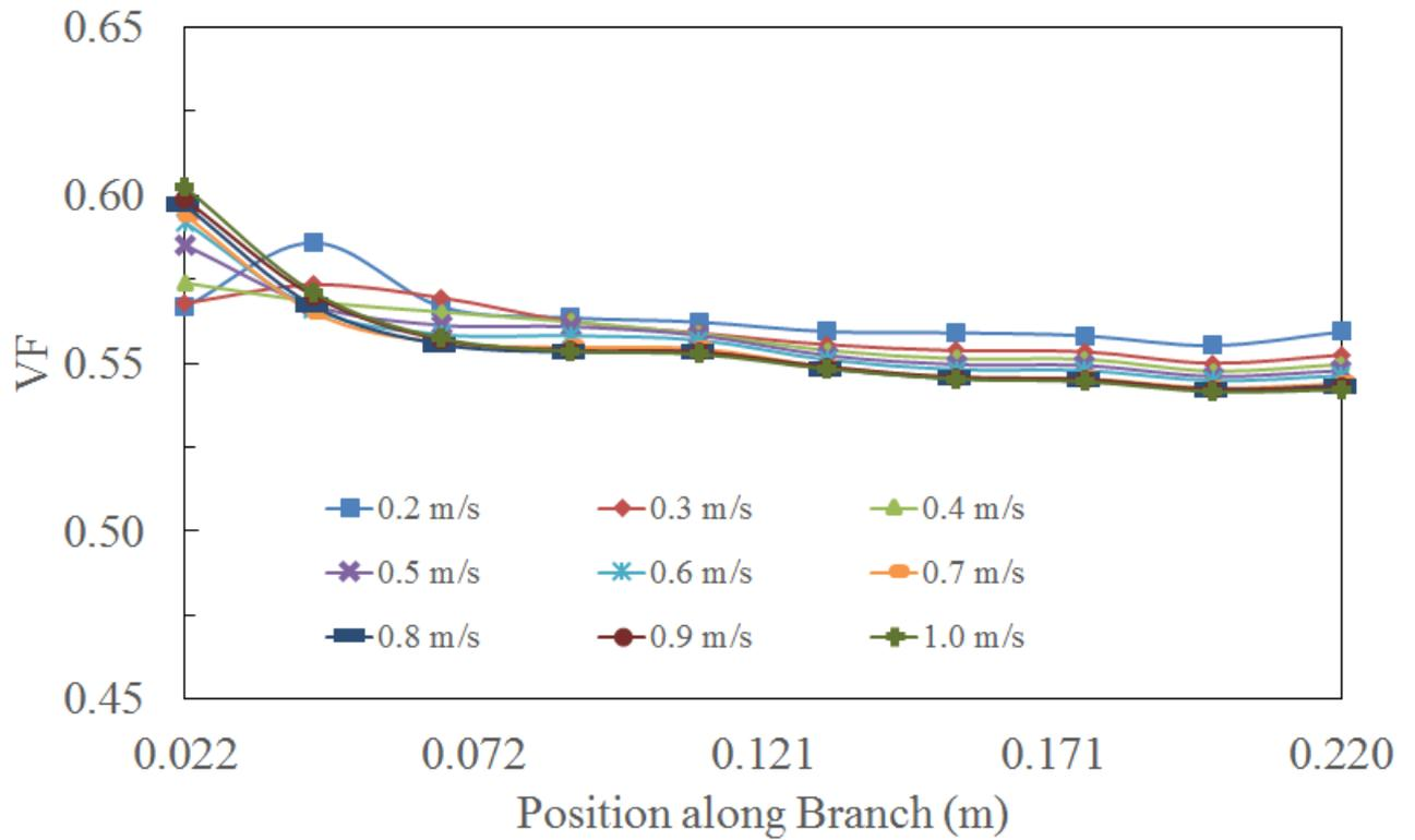
Figure 9: Variation in VF along branch arm for diesel-water pair
