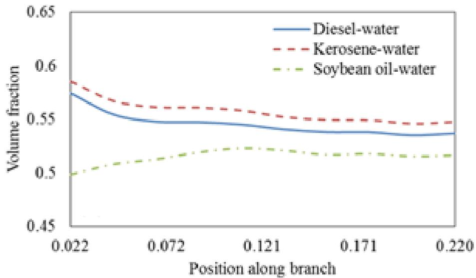
Figure 17: Effect of change in fluid pair on branch arm volume fraction for 11 mm diameter Tee junction
