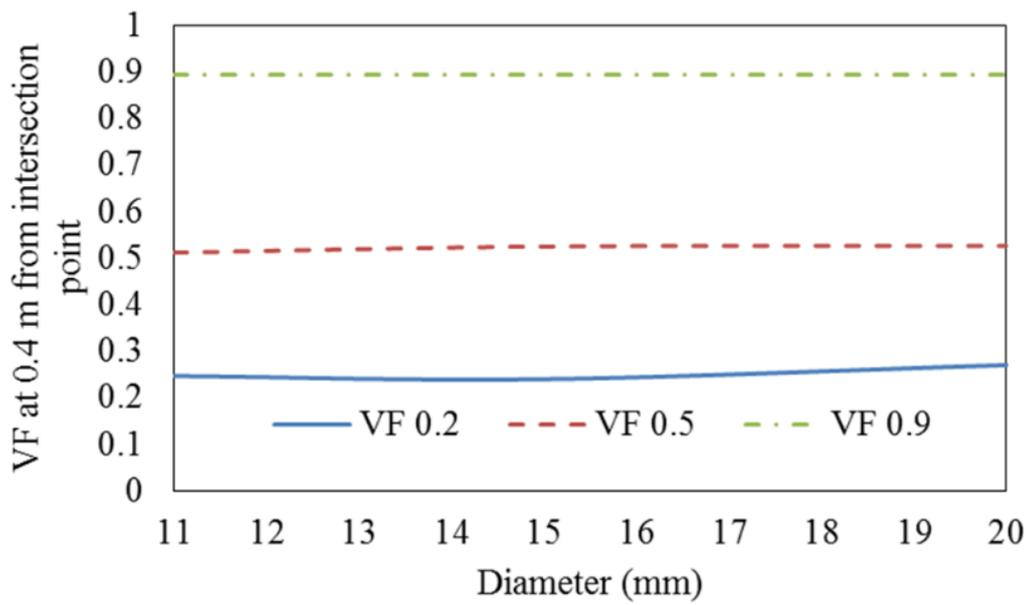
Figure 16: Effect of diameter of Tee junction for soybean oil-water fluid pair
