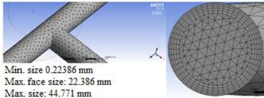
Figure 2: Meshing of the Tee junction
