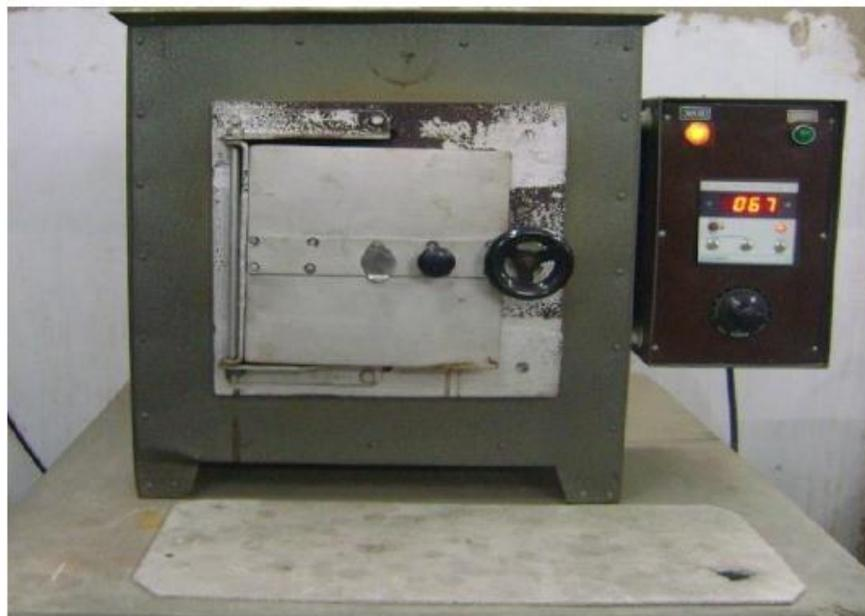
**Plate 4.2 Muffle Furnace for determination of Volatile Matter and Ash Content**
