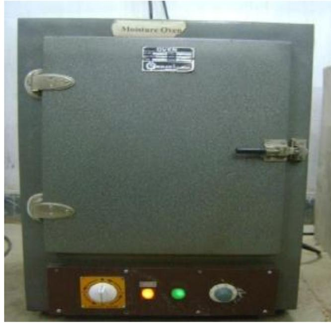
**Plate 4.1 Electric hot air oven**
