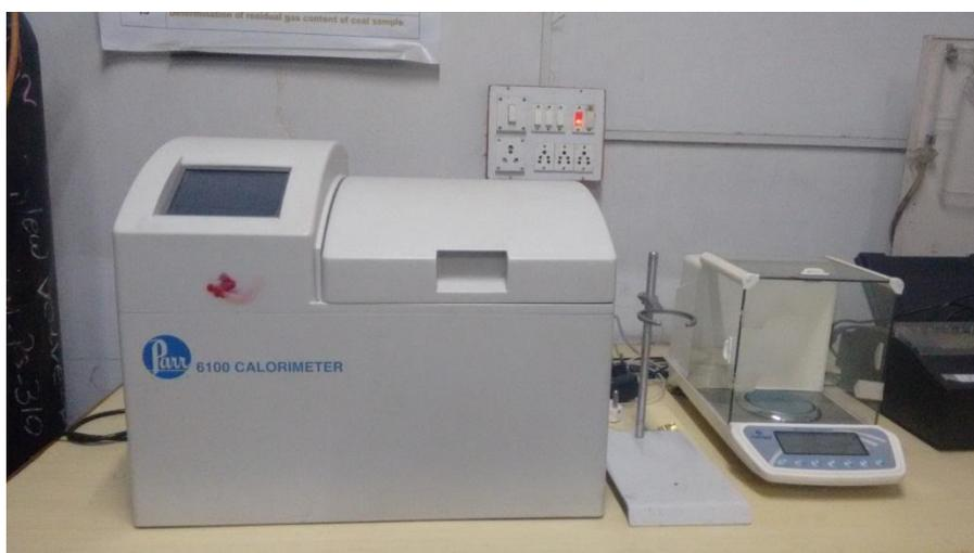
**Plate 4.3 Parr 6100 Calorimeter (Bomb Calorimeter)**
