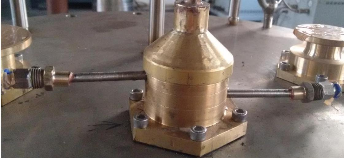
Fig.3.10 Photographic view of Hot end heat exchanger
