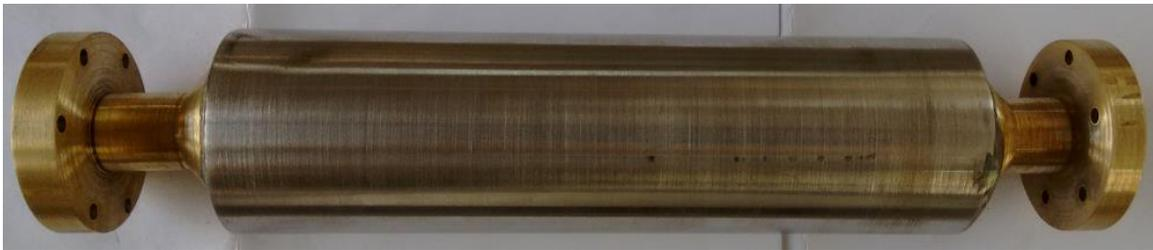
Fig.3.3 Photographic view of Regenerator
