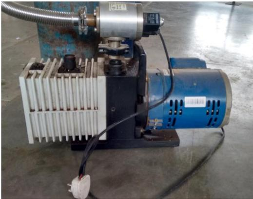
Fig.4.6 Vacuum pumping system
