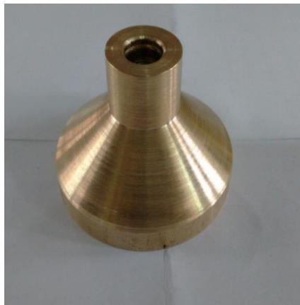
Fig.3.9 Convergent section Hot end heat exchanger
