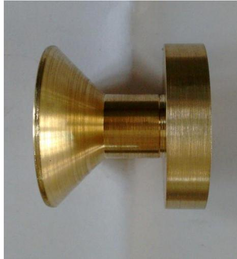
Fig.3.2 (b) Bottom flange of Regenerator
