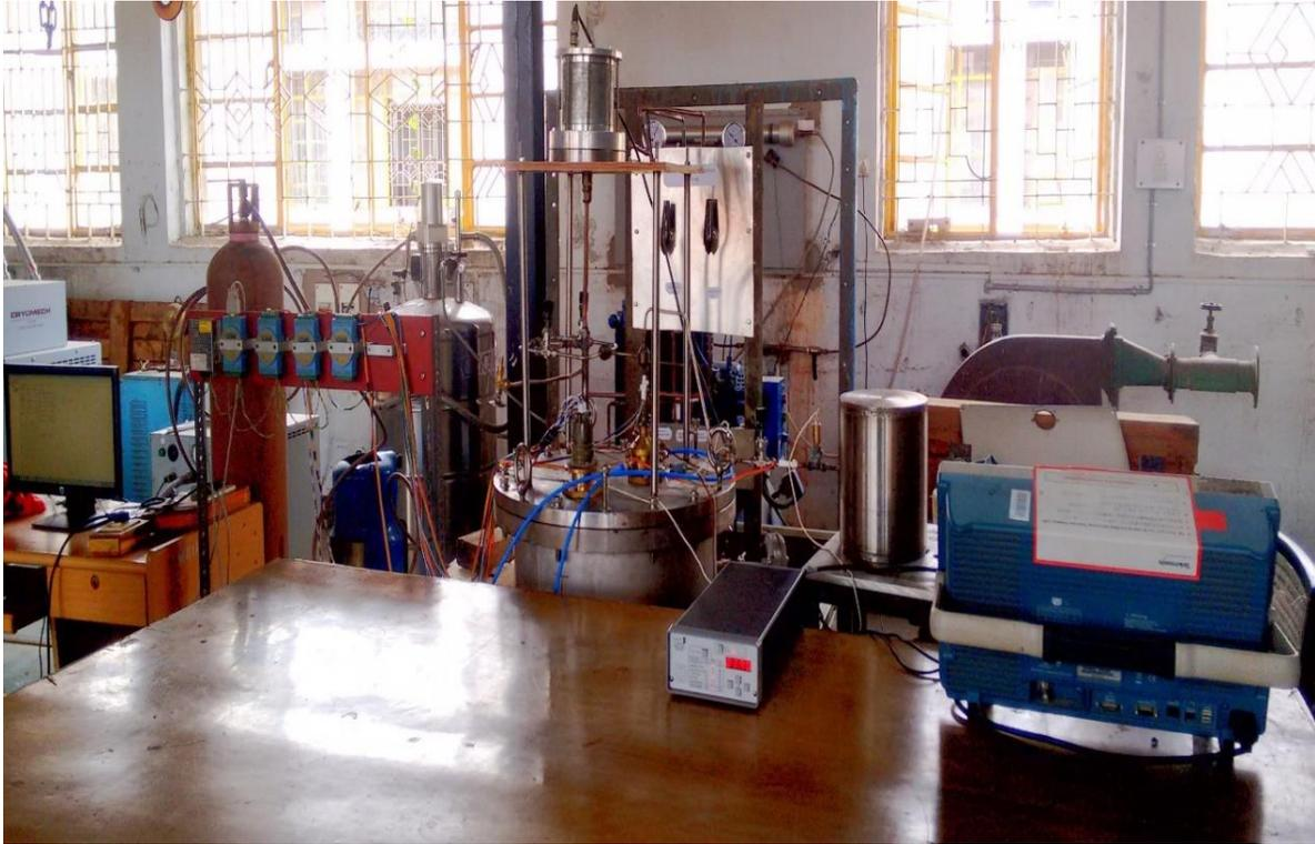
Fig.4.2 Experimental test-rig of Pulse Tube Refrigerator
