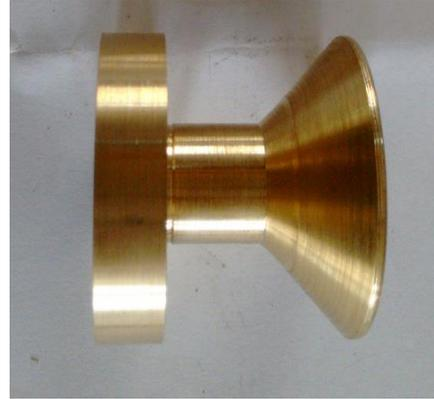
Fig.3.4 (b) Bottom flange of Pulse tube
