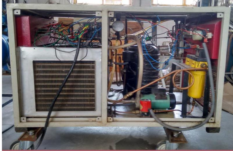
Fig.4.3 Photographic view of reciprocating helium Compressor
