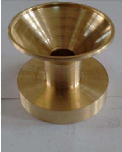
Fig.3.2 (a) Top flange of Regenerator
