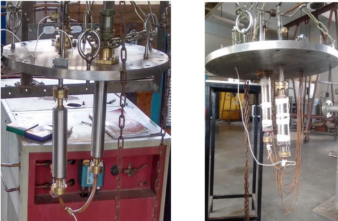
Fig.4.9 Typical assembly of pulse tube refrigerator before and after incorporation of pressure and temperature sensors.
