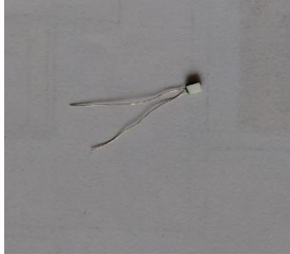
Fig.4.11 A thin film type PT-100 sensor
