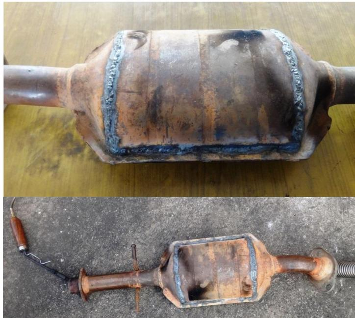
Figure 4.23: Design of tailpipe with zeolite 13x pellets
