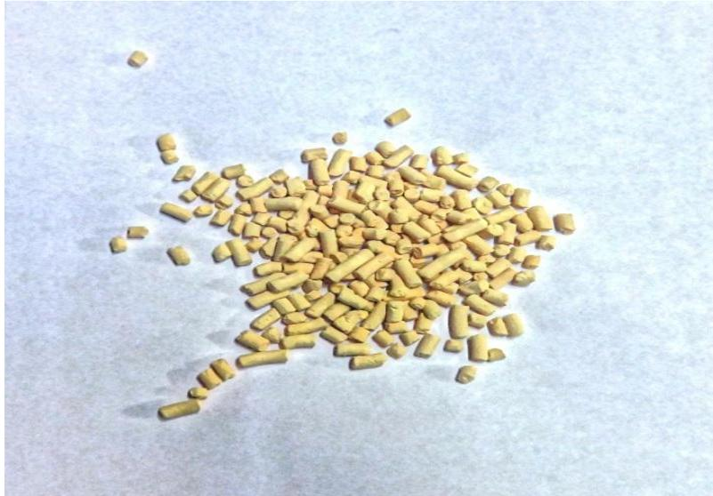
Figure 4.22: Zeolites 13X pellets
