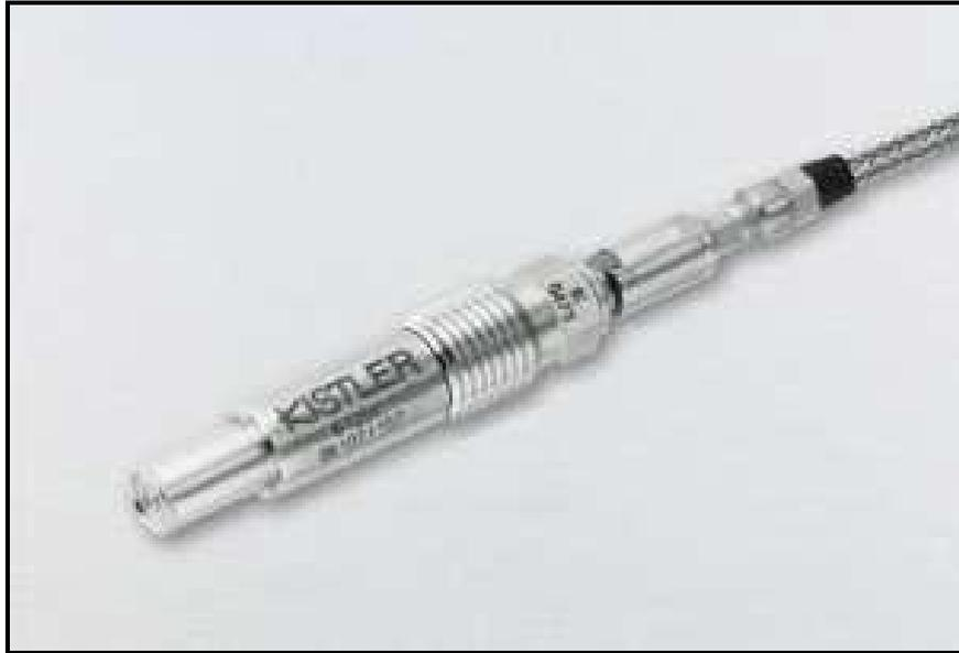
Figure 4.10: Photographic view of the Kistler pressure transducer
