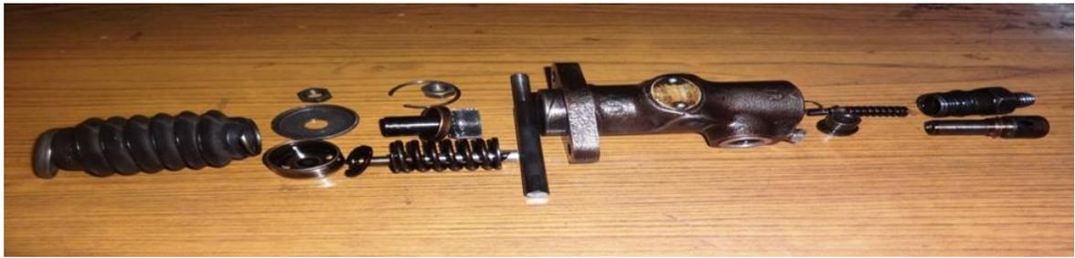
Figure 5.79: Photographic view of all components of the dismantled fuel injection pump
