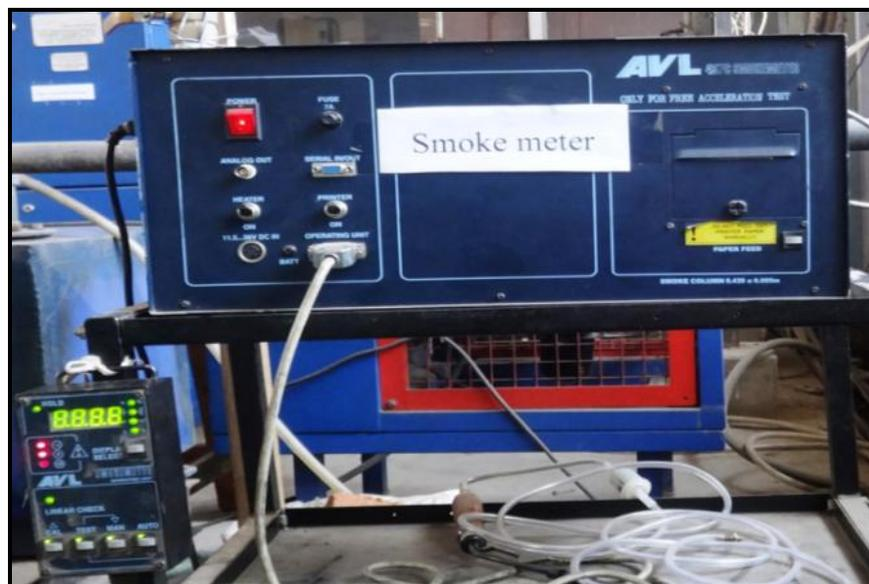
Figure 4.9: Diesel smoke-meter
