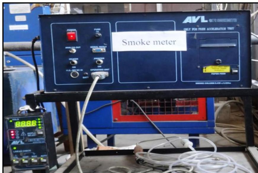
Figure 4.9: Diesel smoke-meter
