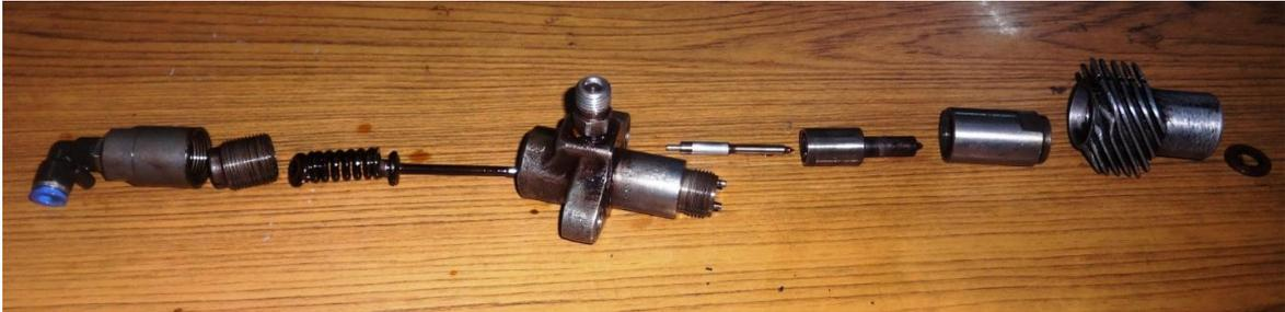
Figure 5.77: Photographic views of the dismantled fuel injector components
