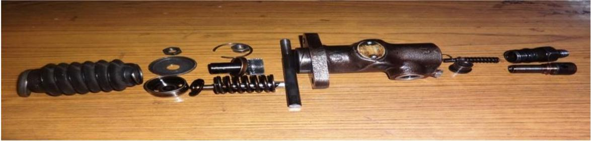
Figure 5.79: Photographic view of all components of the dismantled fuel injection pump
