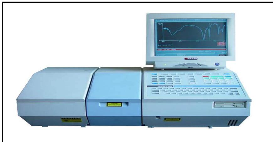
Figure 3.4: Photographic view of spectrophotometer (make: Perkin Elmer Rx1)
