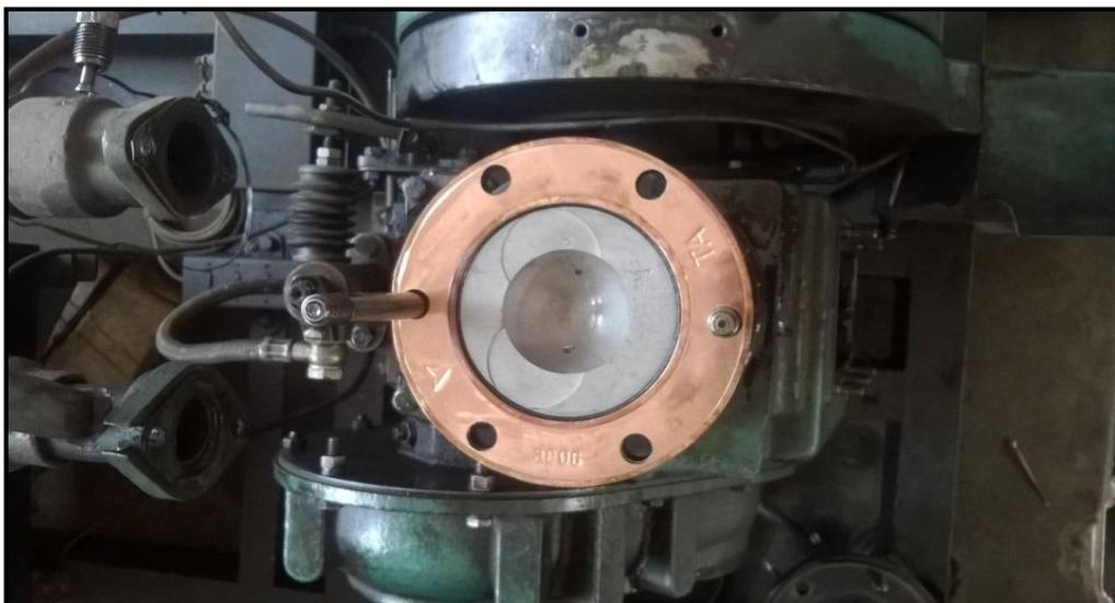
Figure 4.17: Photographic view of an internal jet piston assembled in a diesel engine
