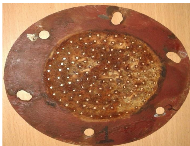
Figure 2.2 Photographic representation of distributor plate
