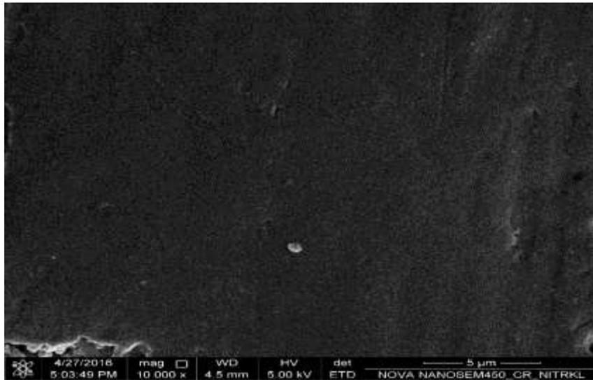
Figure. 17. Micrographs of PP wax at 10000 magnification
