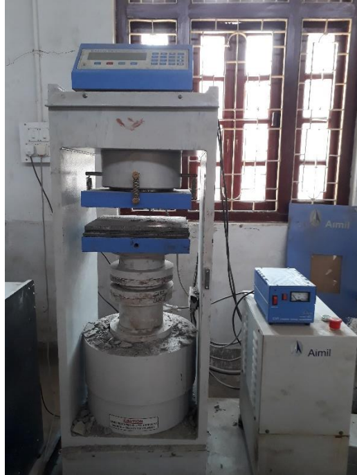
Fig: 3.10- Universal testing machine used for the compression strength test
