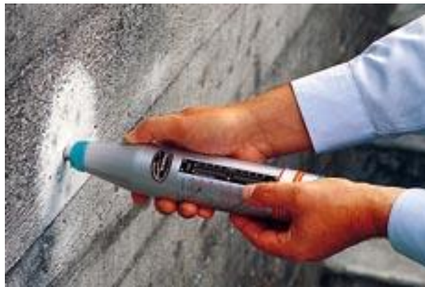
Figure 2.2: Schmidt Concrete Test
