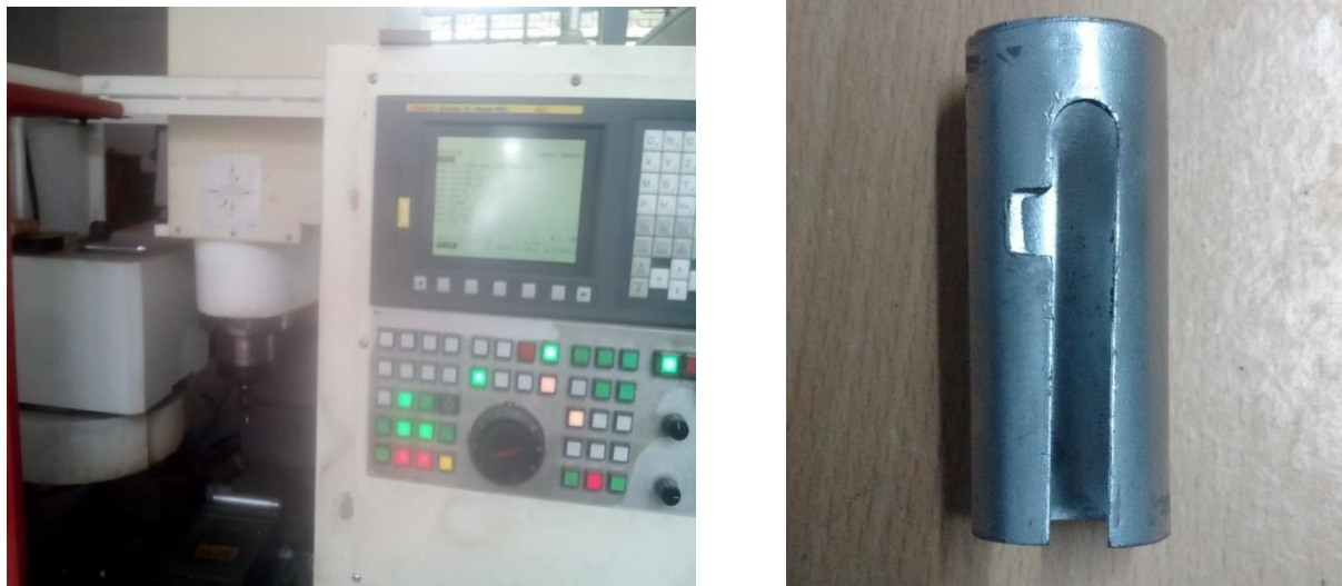
Figure 4.8: Fabrication of Presser on CNC
