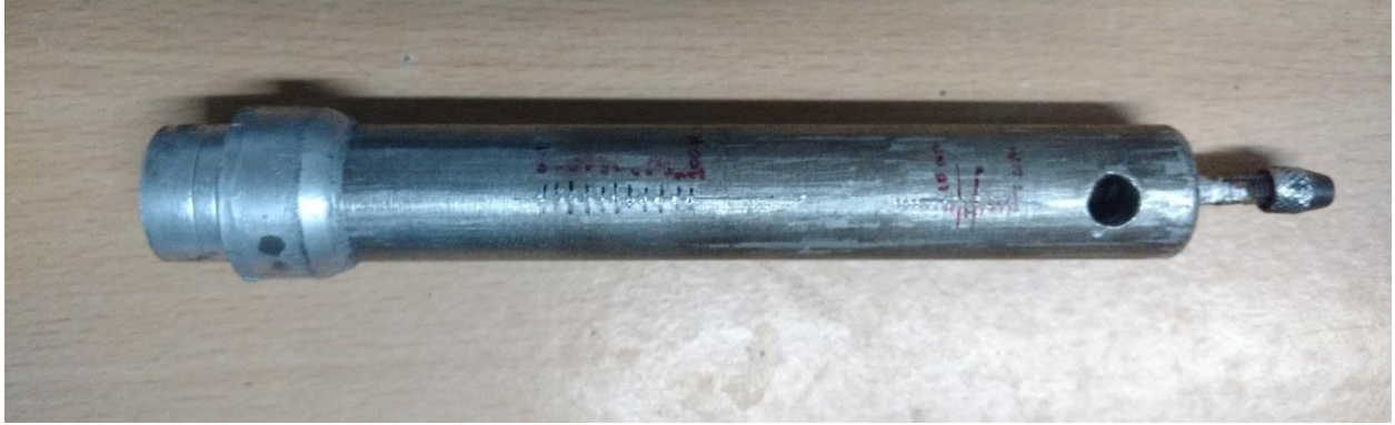
Figure 4.6: Image of fabricated part (Plunger)
