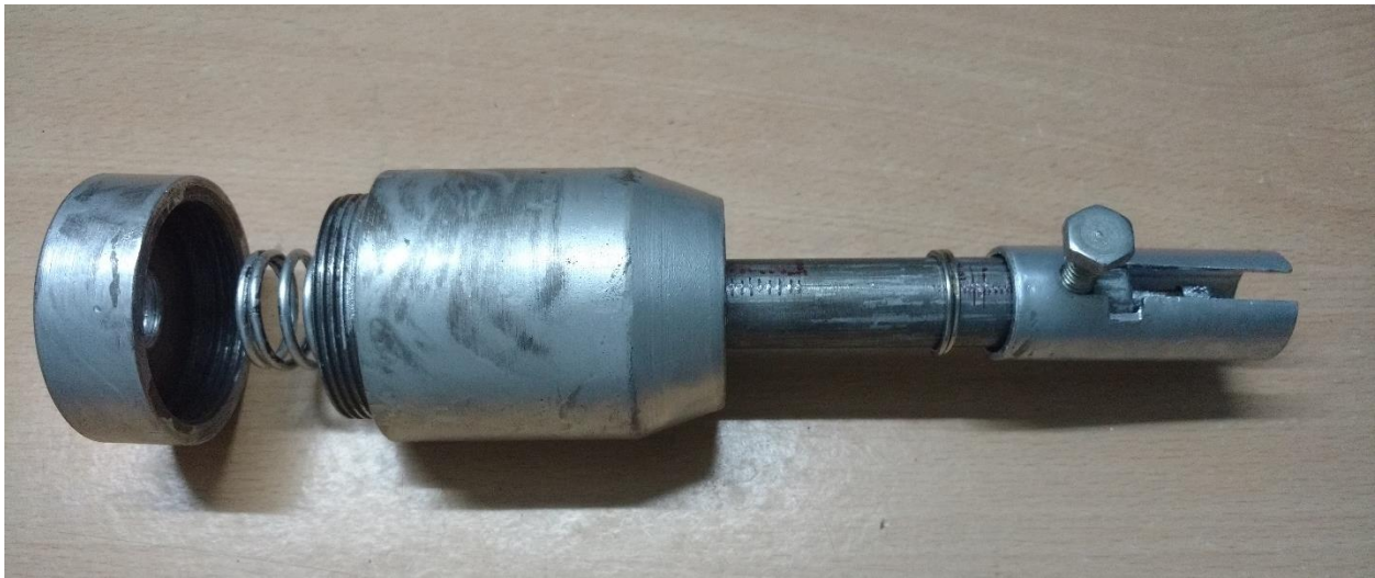
Figure 4.9: Assembly of Needle penetrometer
