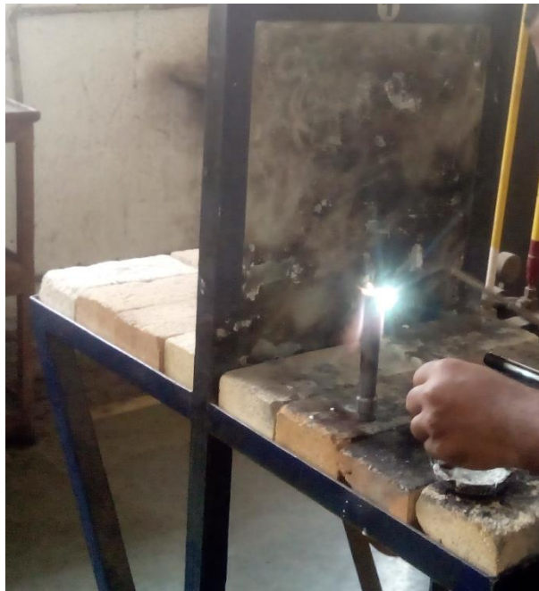
Figure 4.7: Image of Gas welding attaching chuck
