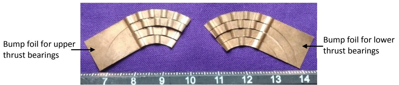
Figure 6.42: Fabricated thrust bump foils using 2<sup>nd</sup> die set for upper and lower thrust bearing.
