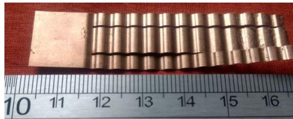
Figure 6.25: Fabricated journal bump foil with 2<sup>nd</sup> die set
