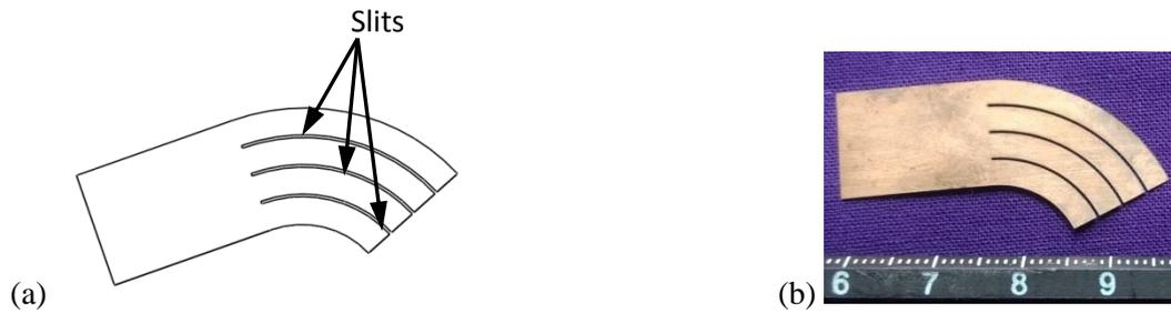
Figure 6.31: Pre-form thrust bump foil: (a) 2D view (b) Fabricated.
