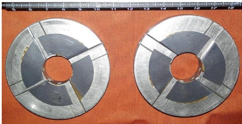
Figure 7.8: MoS<sub>2</sub> coated thrust bearing after test a. upper b. lower.
