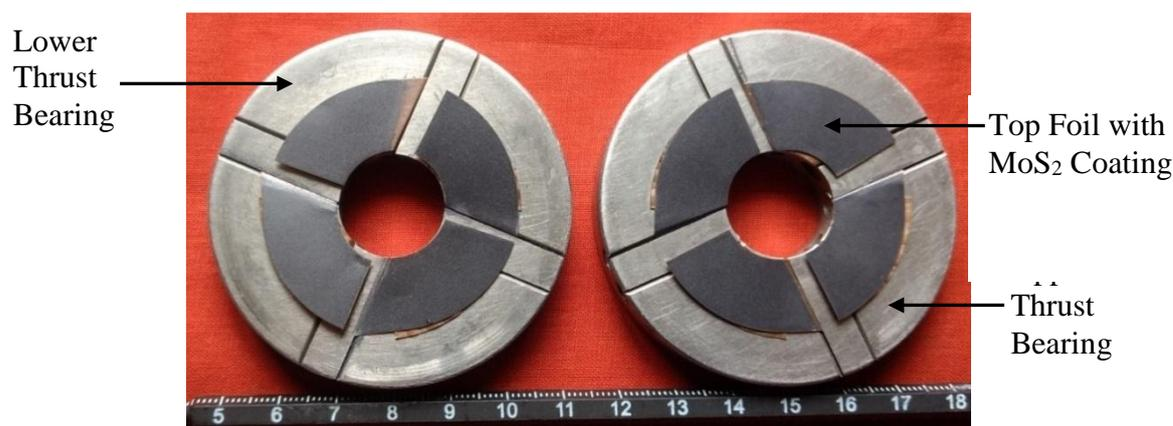
Figure 6.44: Assembled lower and upper gas foil thrust bearing with layer of MoS<sub>2</sub> coating on top foil.
