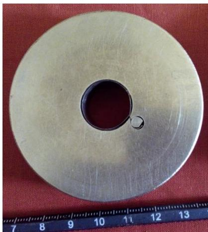
Figure 6.26: Assembly of bump and smooth foil on a single axial hole.
