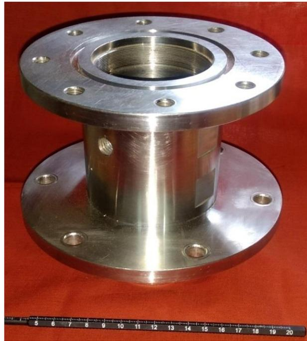
Figure 6.46: Fabricated bearing housing.
