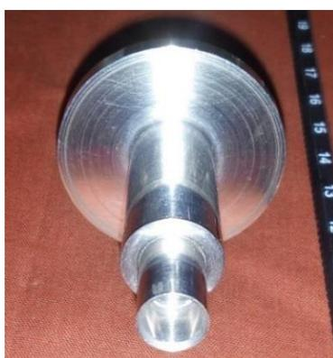
Figure 7.9: Wear on the shaft after the test
