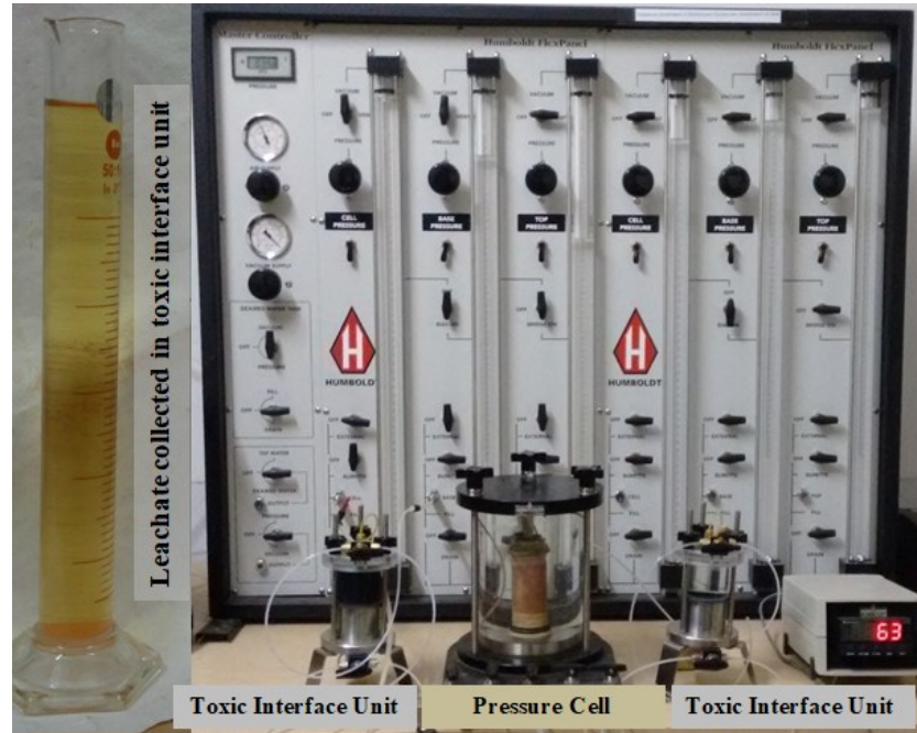
Figure 3.20. Photo of flexible wall permeameter
