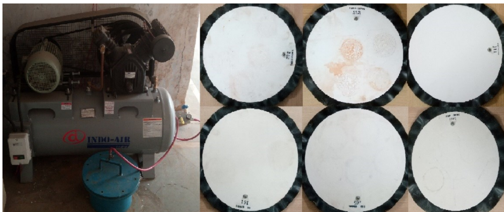
Figure 3.22. Typical photo of pressure plate apparatus with a pressure cell
