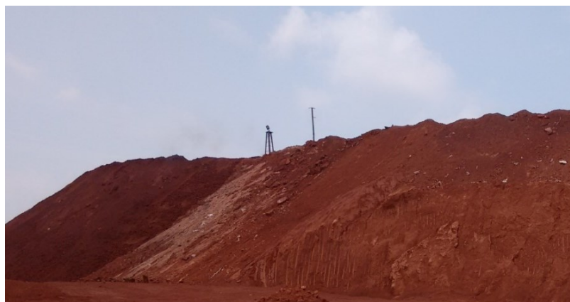
Figure 1.4. Dry disposal system of HINDALCO, Muri (photo by S. Alam)
