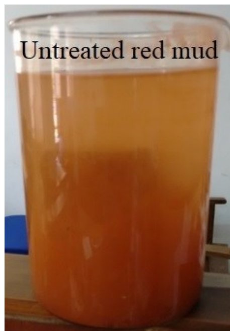
Figure 4.5. Cylindrical dispersive test of un-stabilized NRM (present study)
