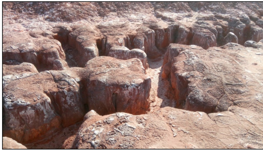
Figure 4.1. A typical picture showing the susceptibility of RM towards water erosion in a RM pond
