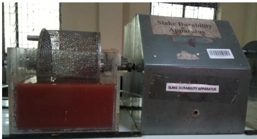
Figure 6.16. Typical photo showing the sample during slake durability test
